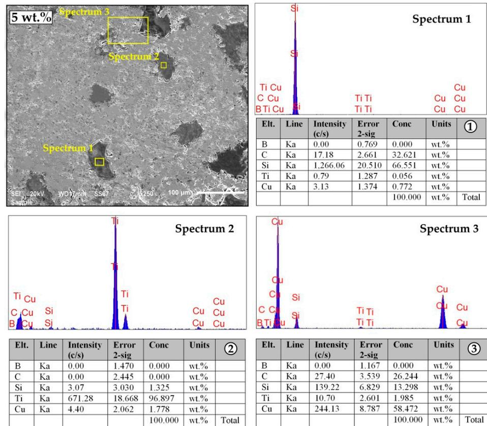
Figure 2. EDX results of the taken from the composites.
