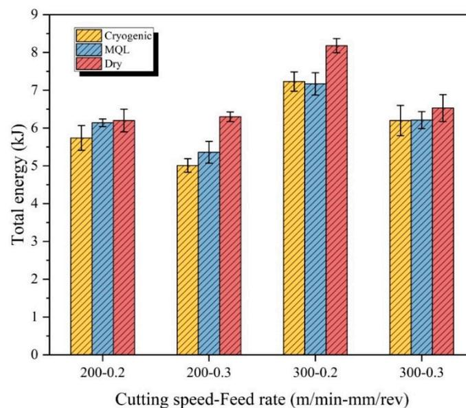
**Figure 9.** Impact of cooling and lubricating on cutting energy consumption.
