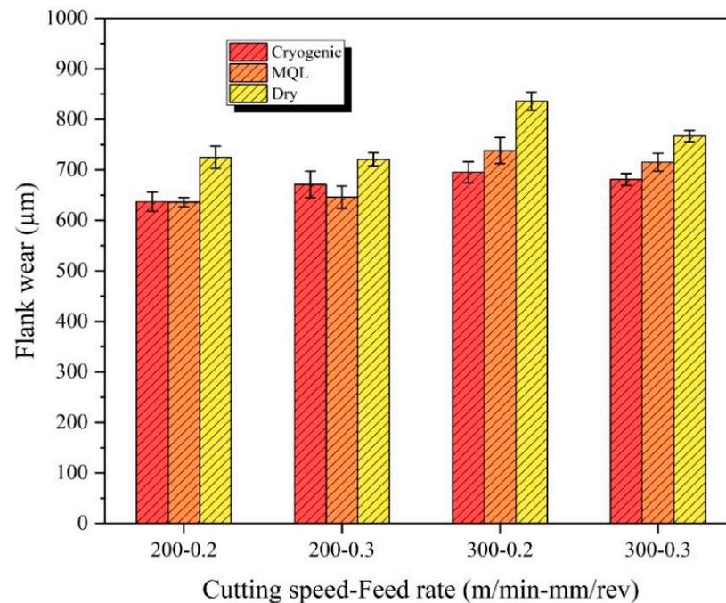
**Figure 3.** Impact of cooling and lubricating effect on flank wear.
