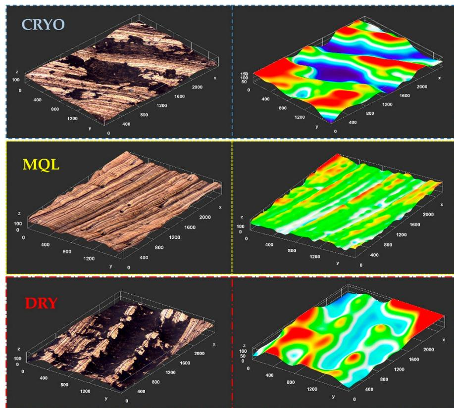
**Figure 7.** Impact of cooling and lubricating on surface texture.
