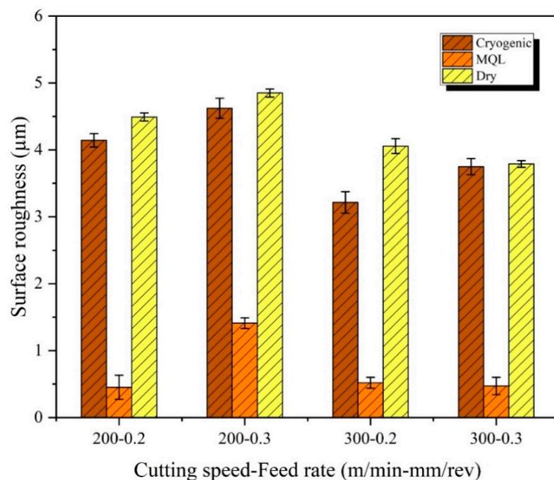
**Figure 6.** Impact of cooling and lubricating on surface roughness.
