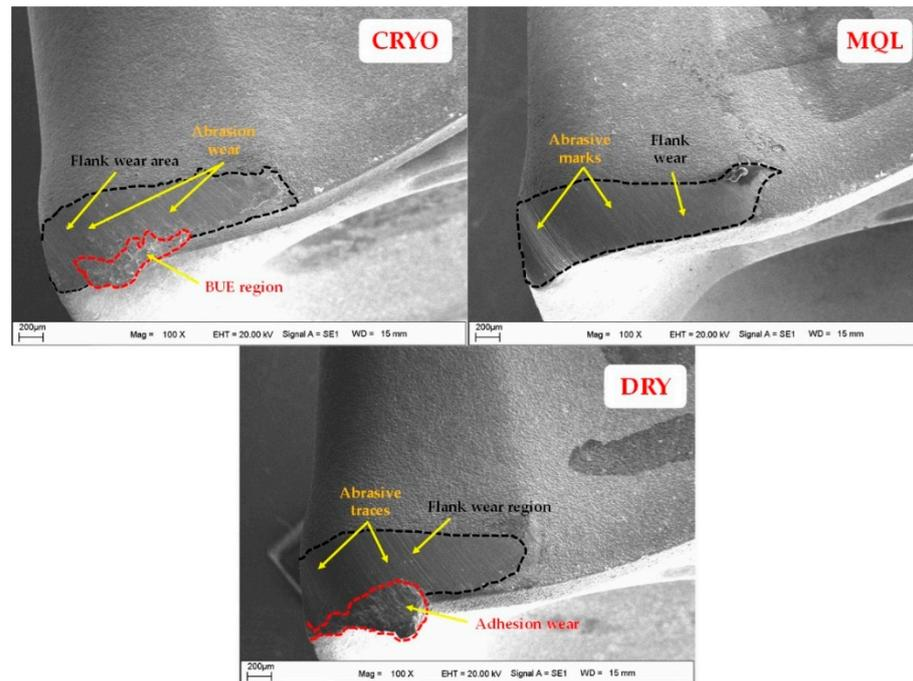
**Figure 4.** Impact of cooling and lubricating on microstructures of flank faces of tool wear.
