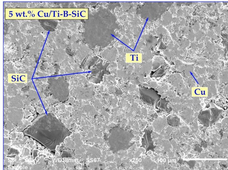
Figure 1. Microstructure of the hybrid composite materials.
