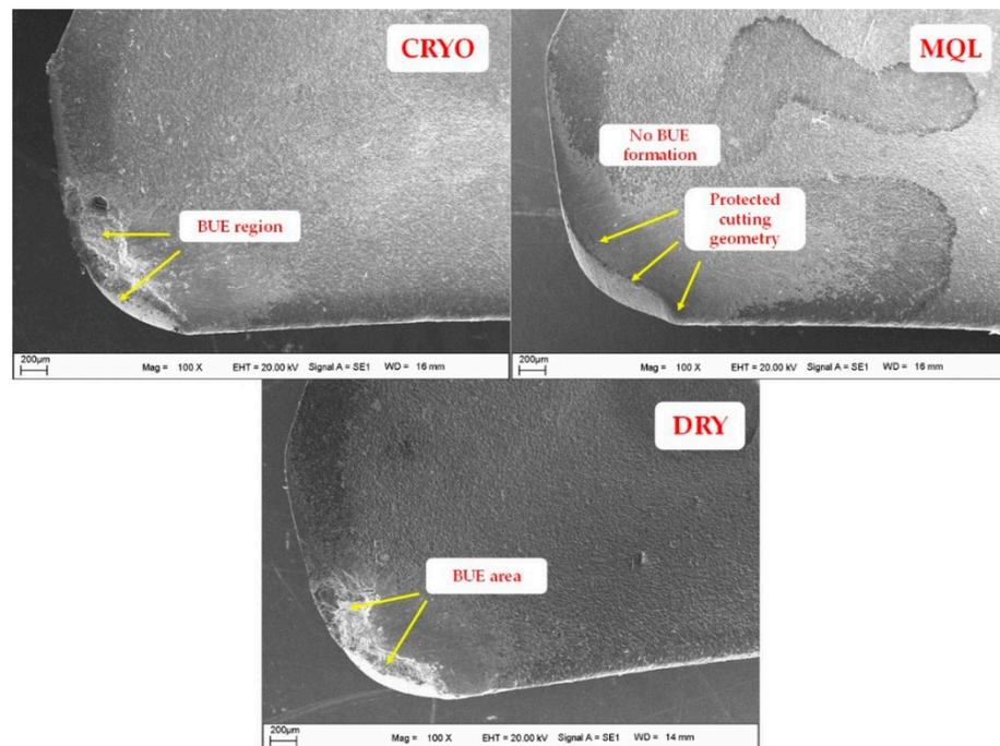
**Figure 5.** Impact of cooling and lubricating on microstructures of rake faces of tool wear.
