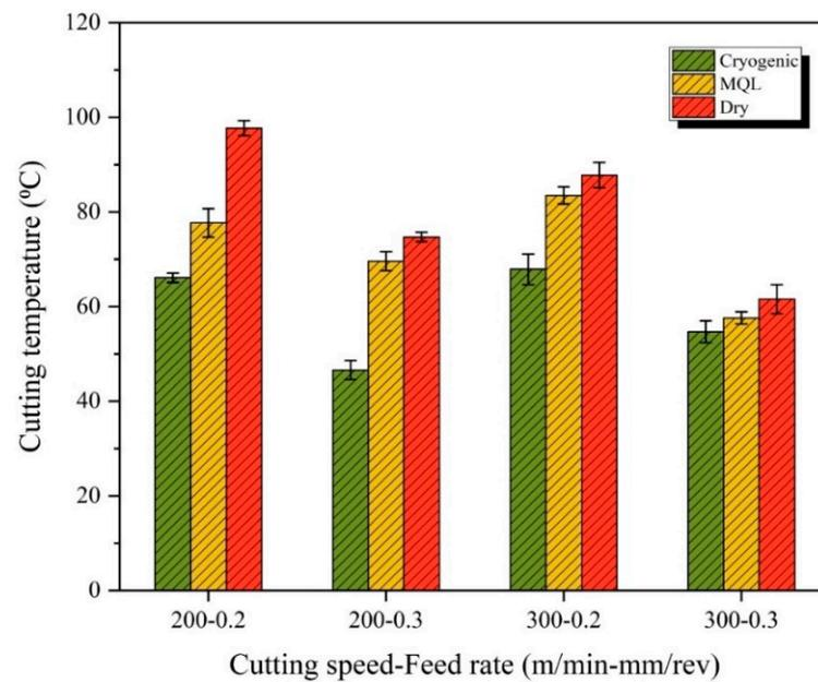
Figure 8. Impact of cooling and lubricating on cutting temperatures.
