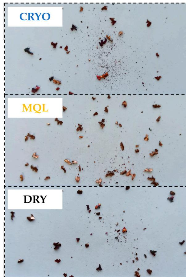
Figure 10. Chips characteristics under different cooling and lubricating conditions.
