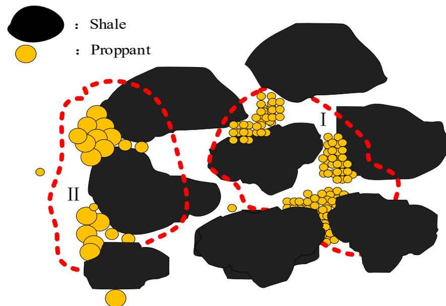
**Figure 5.** Friction and damage mechanism of the proppant. (I) second proppant accumulation; (II) first proppant accumulation.
