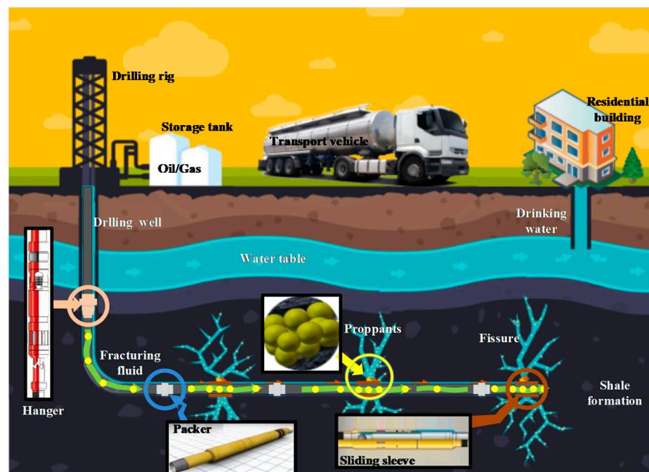
**Figure 1.** Schematic of the hydraulic fracturing process.
