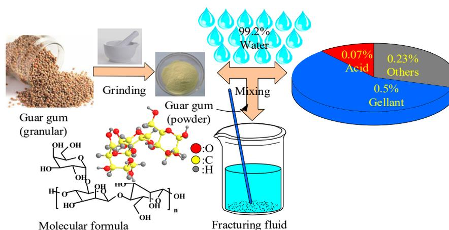
**Figure 3.** Diagram of the water-based fracturing fluid.
