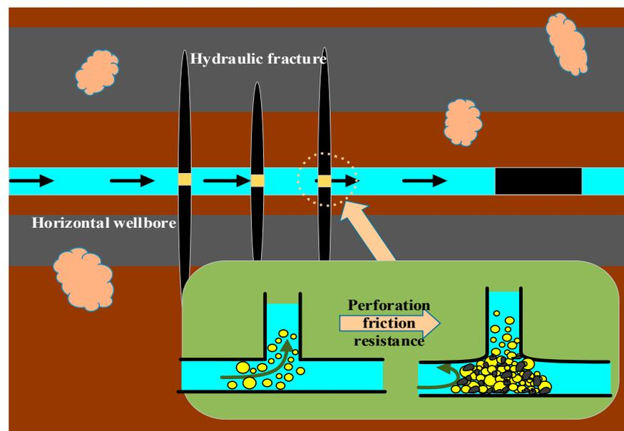
**Figure 6.** The schematic diagram of perforation abrasion.
