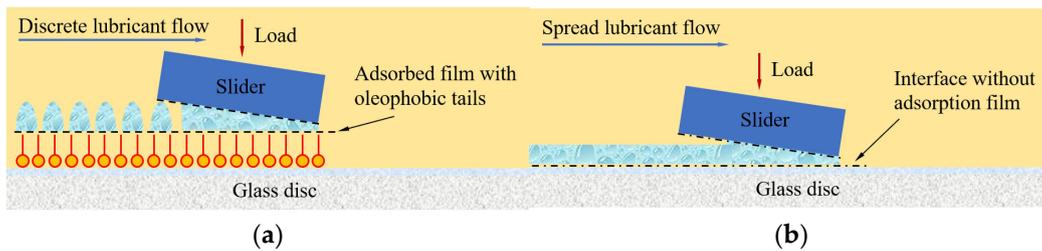
**Figure 9.** Lubricating oil flow model. (a) discrete state; (b) spread state.
