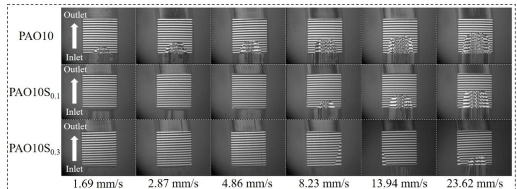
**Figure 7.** Interference diagram of the lubricant film in the contact area of the slider,  $w = 2 \text{ N}$ ,  $q = 2 \mu\text{L}$ .
