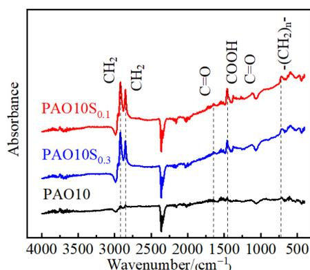
**Figure 17.** Fourier infrared spectroscopy analysis of steel slider surface.
