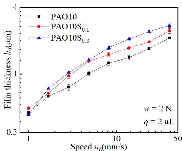
**Figure 8.** The curve of minimum oil film thickness with speed.
