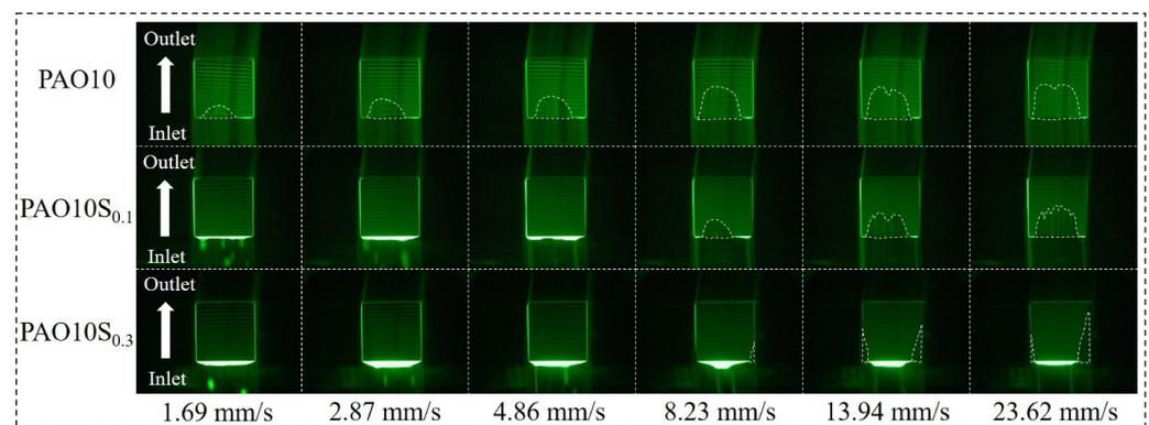
**Figure 5.** Fluorescence images of the oil reservoir at the entrance of the slider with speed,  $w = 2$  N,  $q = 2$   $\mu$ L. (Note that the region of starvation is highlighted by dotted lines for clarify).
