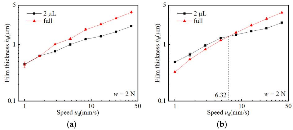
**Figure 11.** Variations of minimum oil film thickness with speed under different oil supply. (a) PAO10; (b) PAO10S<sub>0.1</sub>.
