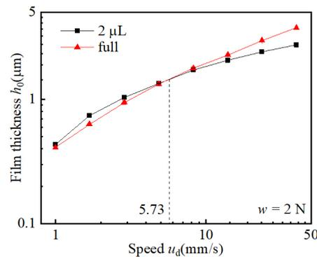
**Figure 14.** Variations of minimum oil film thickness with speed under a different oil supply, PAO10S<sub>0.3</sub>.
