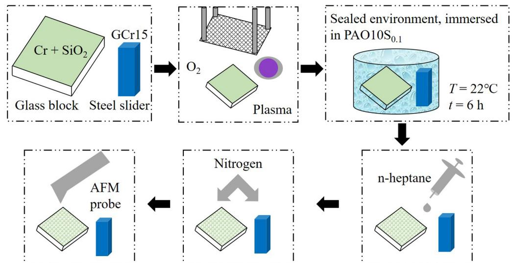
**Figure 15.** Sample preparation and detection process.
