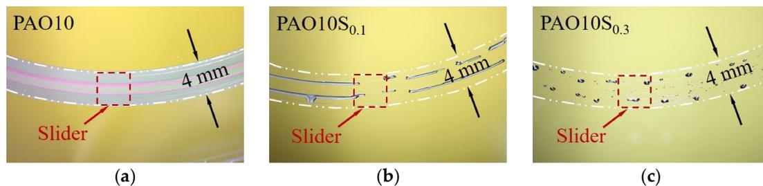
**Figure 4.** Lubricant distribution pattern on glass disc track surface,  $w = 2$  N,  $q = 2$   $\mu$ L. (a) PAO10, (b) PAO10S<sub>0.1</sub> and (c) PAO10S<sub>0.3</sub>.
