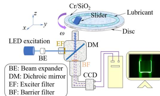
**Figure 2.** Schematic of fluorescence measurement system.
