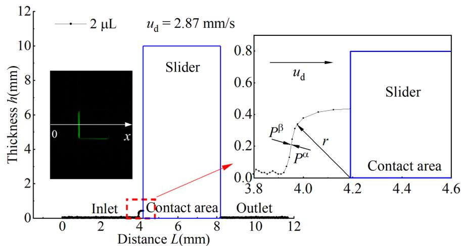
**Figure 12.** Accumulation of lubricant at the inlet of slider,  $w = 2 \text{ N}$ .
