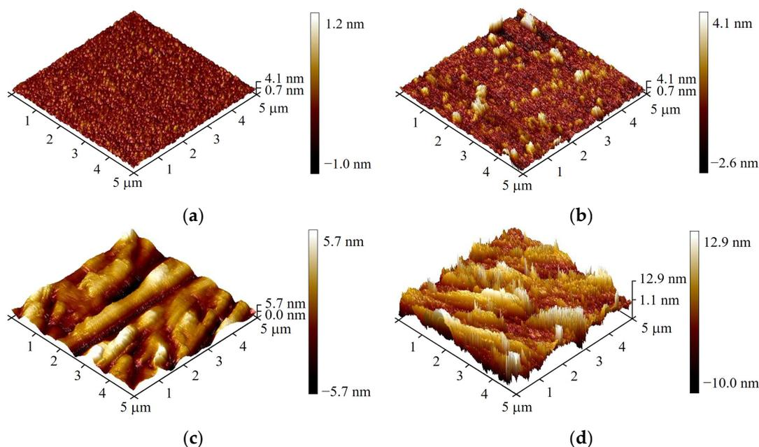
**Figure 16.** AFM surface morphology measurement results. (a) original glass block; (b) adsorbed glass block; (c) original steel slider; (d) adsorbed steel slider.
