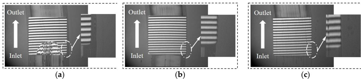
**Figure 6.** The distribution of the oil on the slider side edge,  $w = 2$  N,  $q = 2$   $\mu$ L,  $u_d = 4.86$  mm/s. (a) PAO10, (b) PAO10S<sub>0.1</sub> and (c) PAO10S<sub>0.3</sub>.
