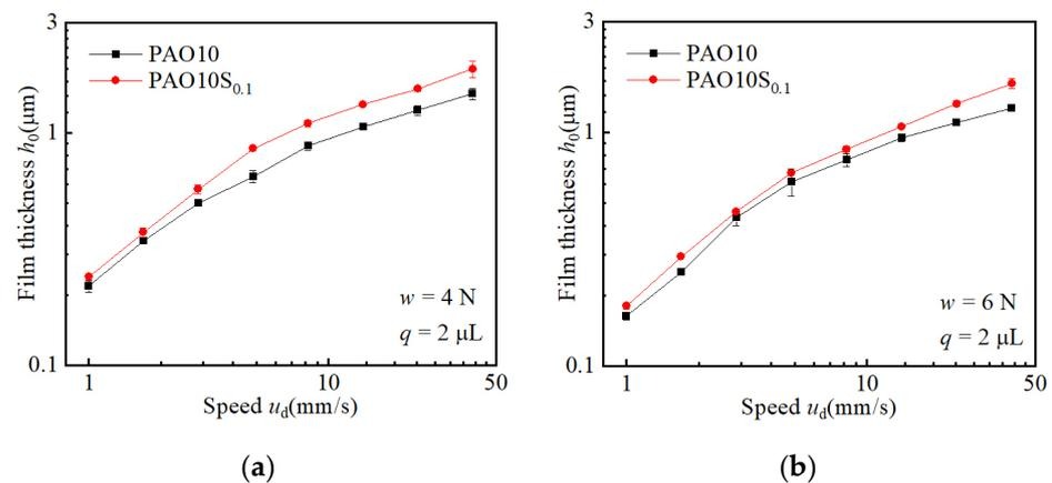
**Figure 10.** Variations of minimum oil film thickness with speed. (a)  $w = 4\text{ N}$ ; (b)  $w = 6\text{ N}$ .
