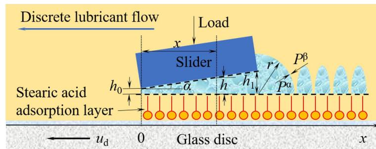
Figure 13. Accumulation mode of lubricant at the inlet of slider.
