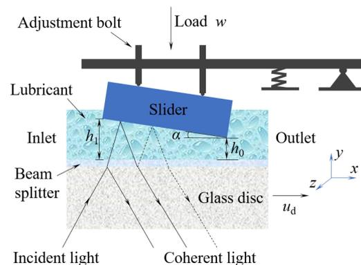
**Figure 1.** Schematic illustration of the optical slider-bearing test rig.
