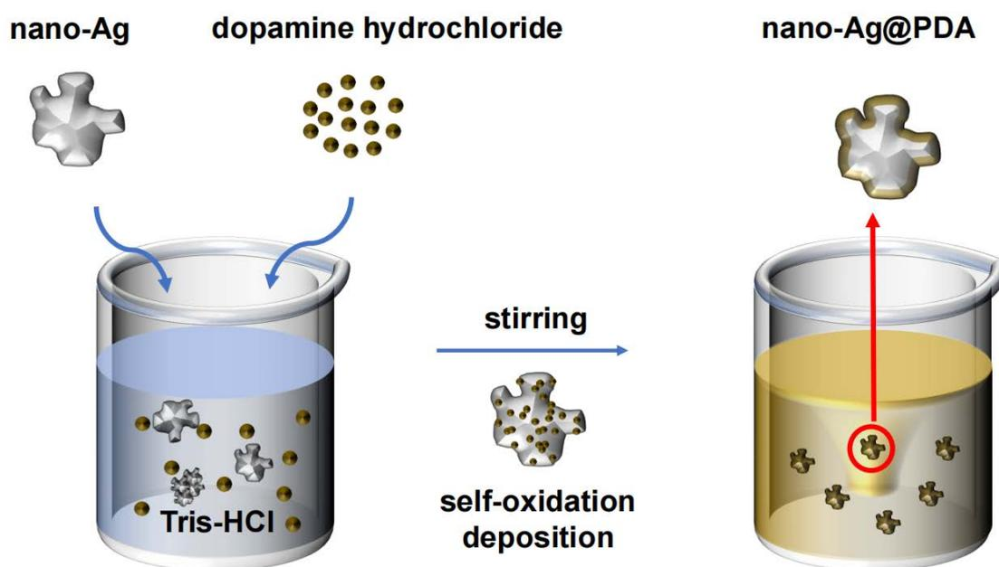
**Figure 1.** Schematic representation of the synthesis of Ag@PDA.
