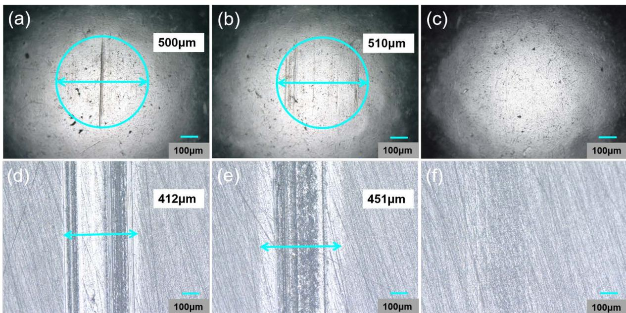
**Figure 8.** Optical images of wear scar diameter of steel balls (a) pure PAO6; (b) oil with 0.25 wt% Ag; (c) oil with 0.25 wt% Ag@PDA and wear scar width of resin matrix (d) pure PAO6; (e) oil with 0.25 wt% Ag; (f) oil with 0.25 wt% Ag@PDA.
