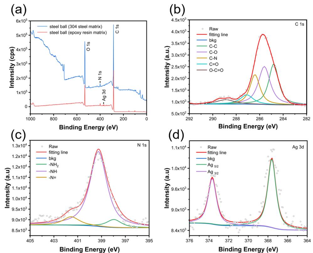
Figure 14. XPS spectra of steel ball surface after friction with (a) Ag@PDA 304 steel and Ag@PDA epoxy resin; high-resolution XPS spectra in the core level (b) C 1s, (c) N 1s and (d) Ag 3d regions for Ag@PDA epoxy resin.
