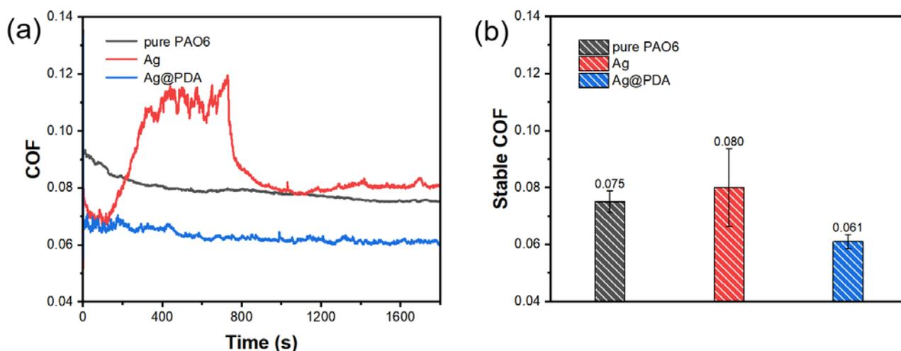
**Figure 7.** (a) Coefficients of friction for samples with different additives under test conditions and (b) stable coefficients of friction for samples with different additives under test conditions.
