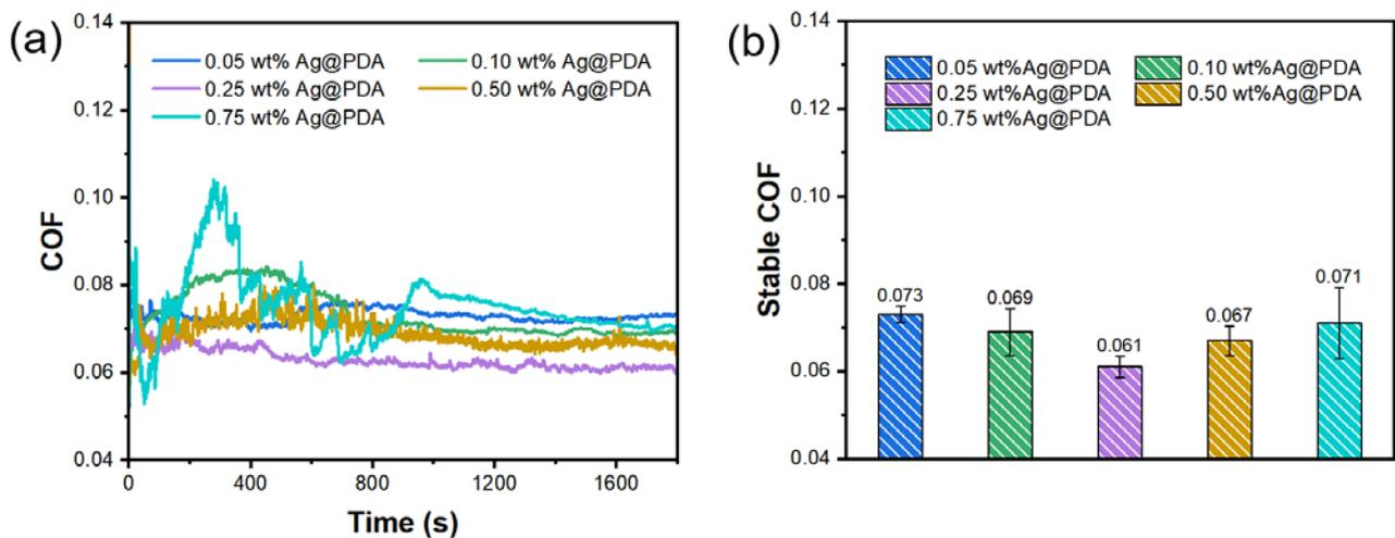
**Figure 9.** (a) Coefficients of friction for samples with different concentrations of Ag@PDA additives under test conditions and (b) stable coefficients of friction for samples with different concentrations of Ag@PDA additives under test conditions.
