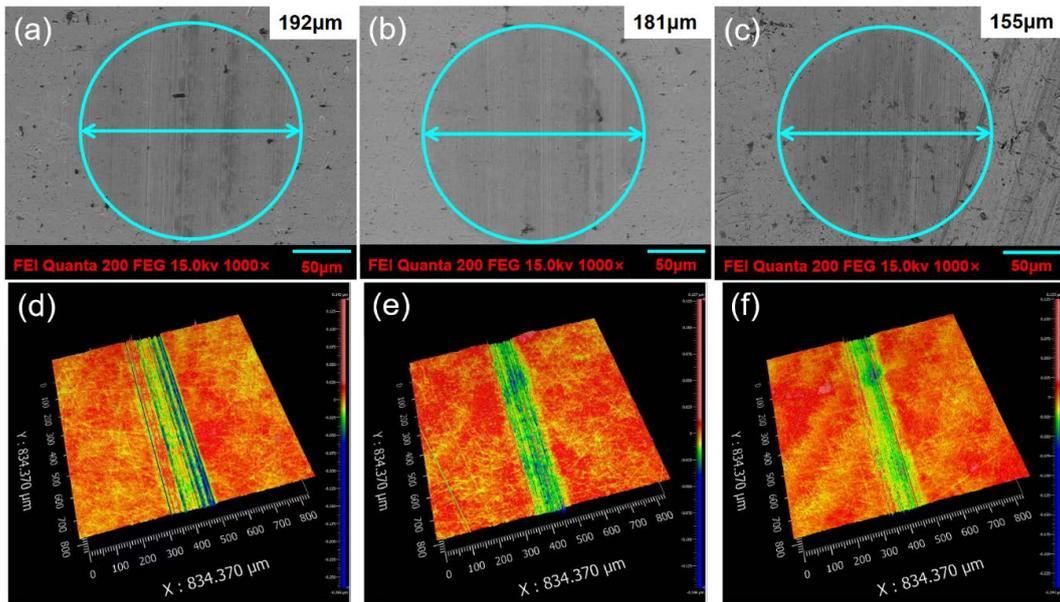
Figure 13. SEM micrographs of steel balls and 3D morphologies of different worn surfaces of 304 steel matrix using: (a,d) pure PAO6; (b,e) PAO6 with 0.25 wt% Ag; (c,f) PAO6 with 0.25 wt% Ag@PDA.
