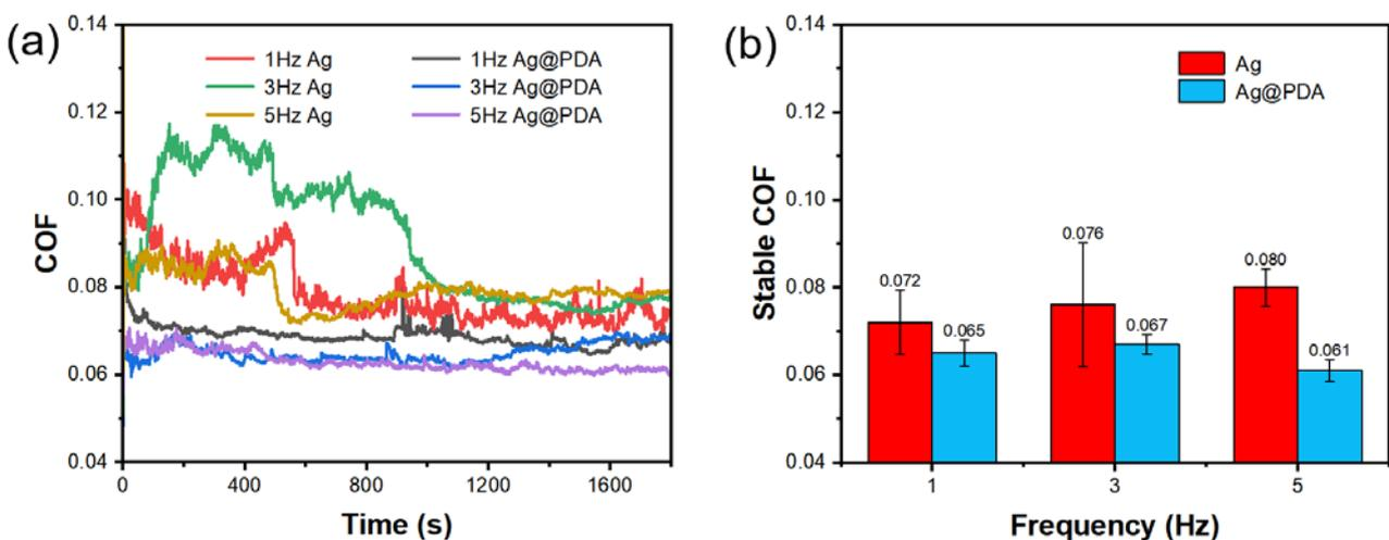
**Figure 11.** (a) Coefficients of friction for samples with different frequencies under test conditions and (b) stable coefficients of friction for samples with different frequencies under test conditions.
