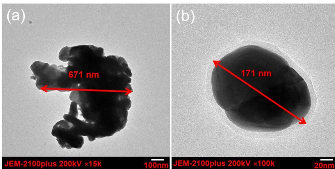
**Figure 4.** TEM micrographs of Ag (a) unmodified; (b) modified.
