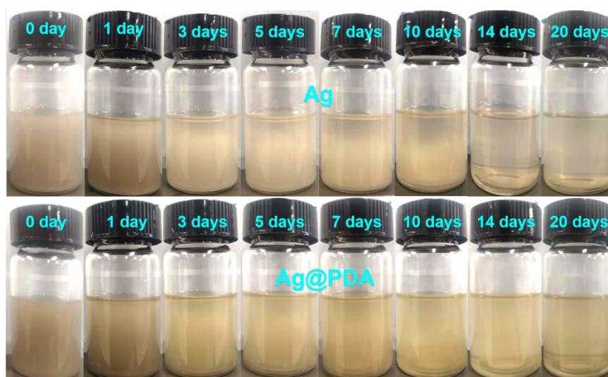
**Figure 5.** Dispersion state of nanoparticles in oil phase when standing for different times.
