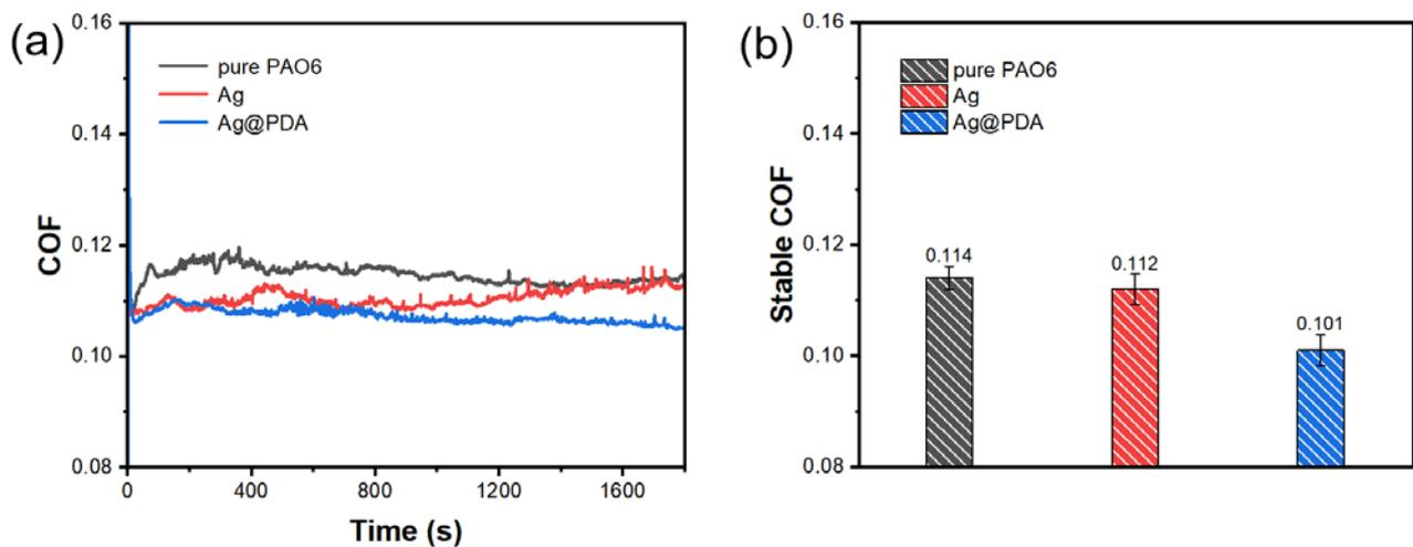
**Figure 12.** (a) Coefficients of friction for samples with 304 steel matrix and (b) stable coefficients of friction for samples with 304 steel matrix.
