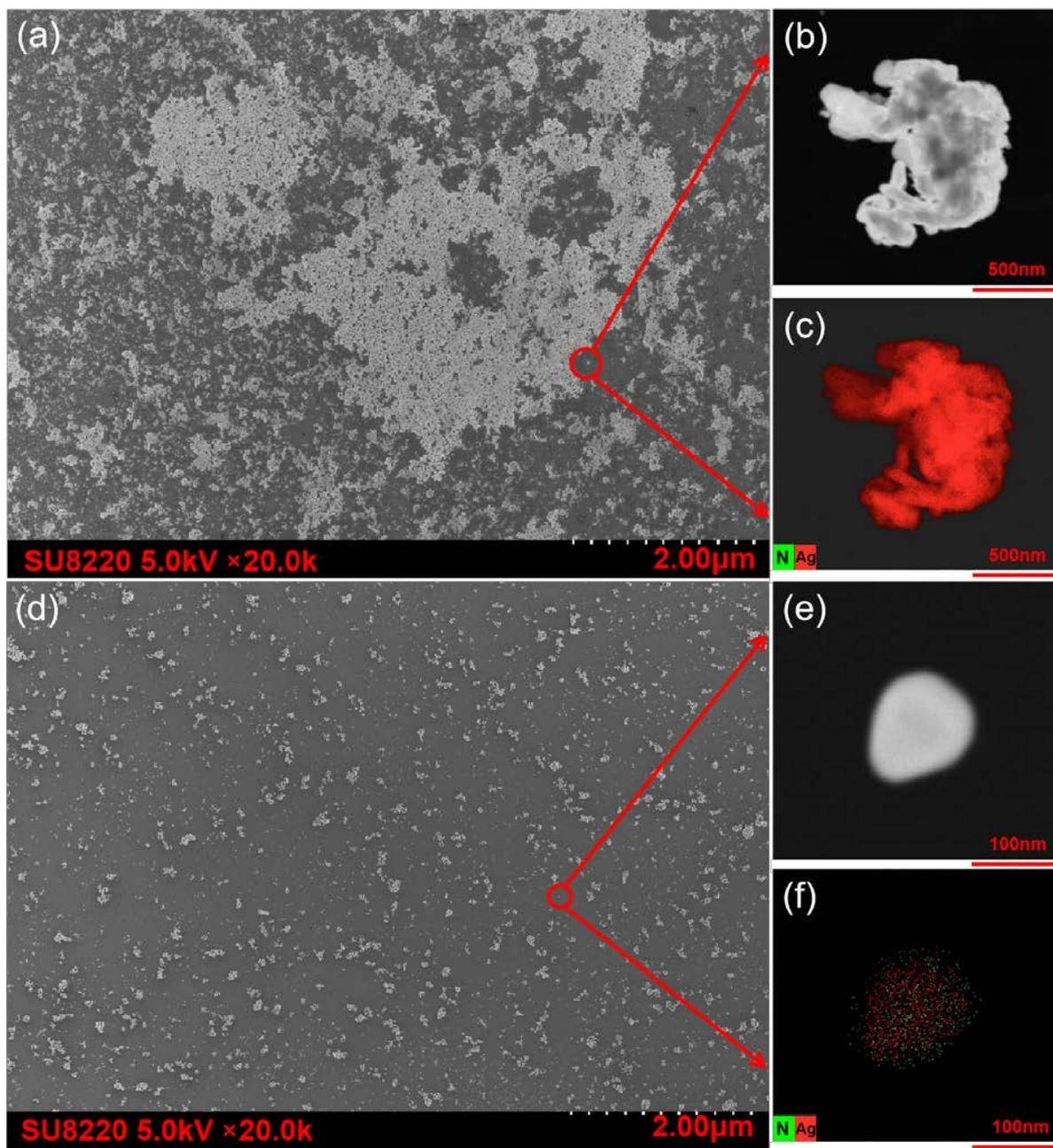
**Figure 3.** (a) SEM micrograph of unmodified Ag; (b,c) TEM-EDS maps of unmodified Ag; (d) SEM micrograph of modified Ag; (e,f) TEM-EDS maps of modified Ag.
