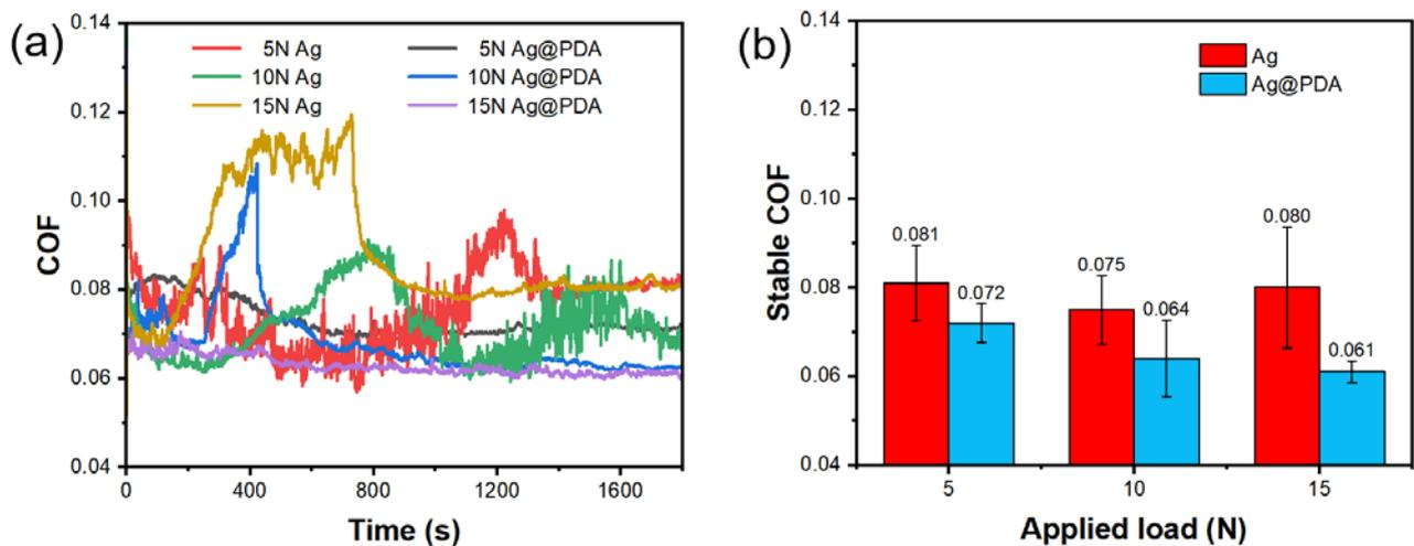
**Figure 10.** (a) Coefficients of friction for samples with different applied loads under test conditions and (b) stable coefficients of friction for samples with different applied loads under test conditions.
