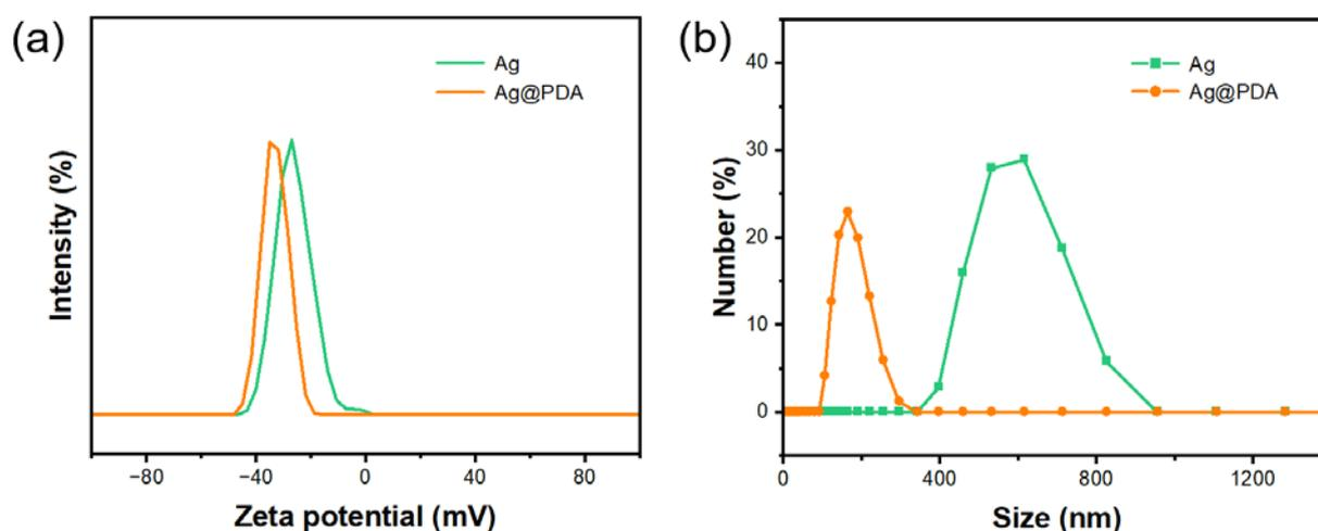
**Figure 6.** (a) Zeta potential of samples unmodified/modified; (b) particle size distribution of samples unmodified/modified.
