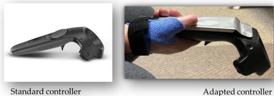
Figure 3. Adaptation to the HTC Vive pro controller.
