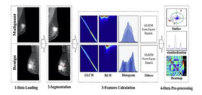
Figure 4. The radiomics workflow of acquisition and pre-processing [46].
