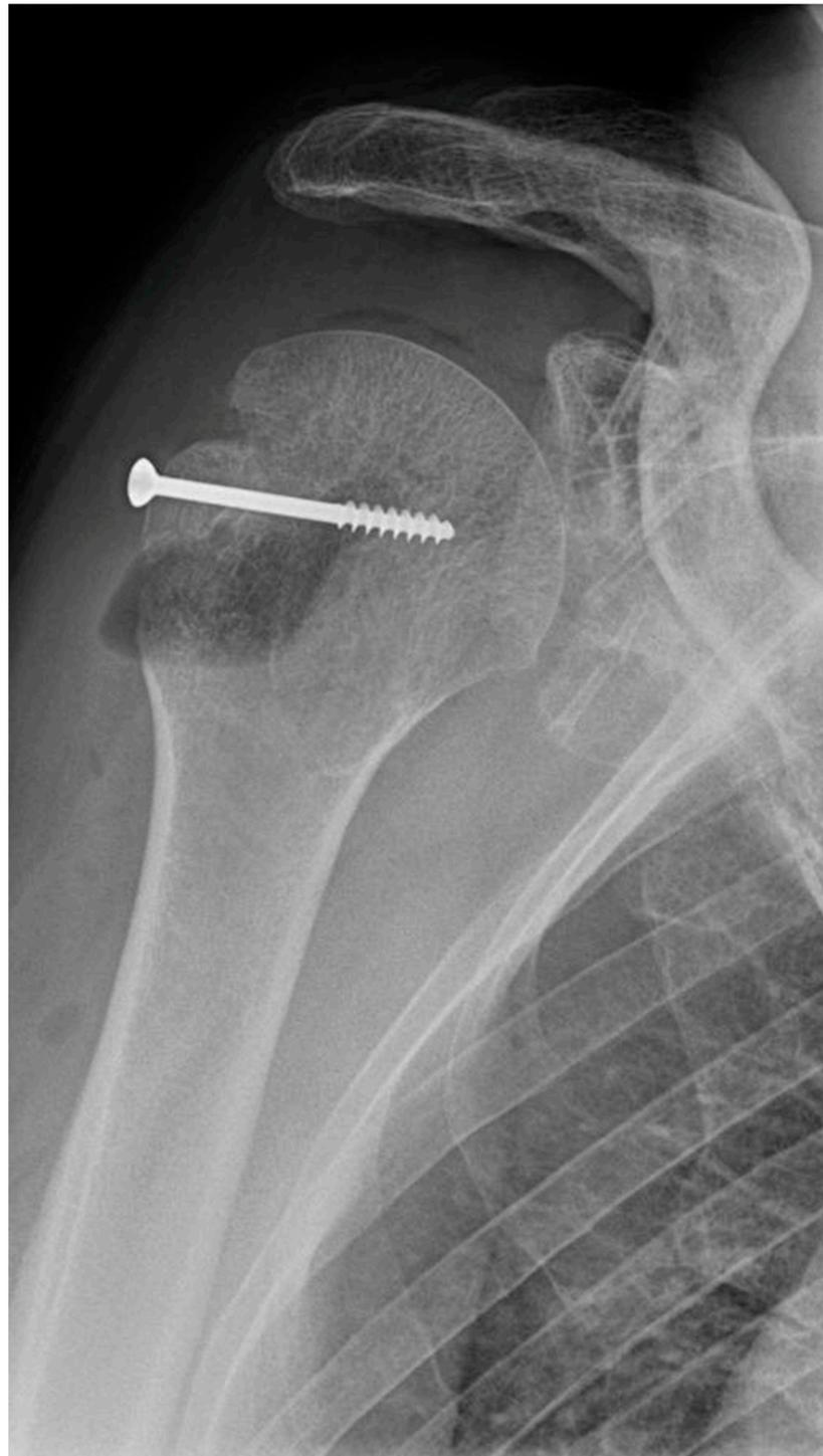
**Figure 3.** Material failure of MAGNEZIX<sup>®</sup> CS screws used for osteosynthesis in a glenoid fracture after anterior shoulder dislocation.
