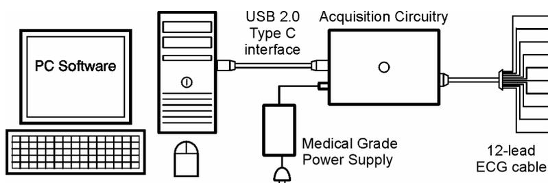
**Figure 3.** The Kenshin device connectivity diagram.
