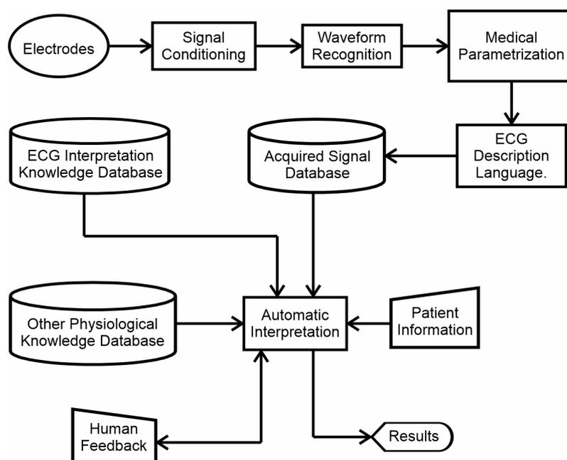
**Figure 10.** A suggested approach for integrating an electrocardiography expert system.
