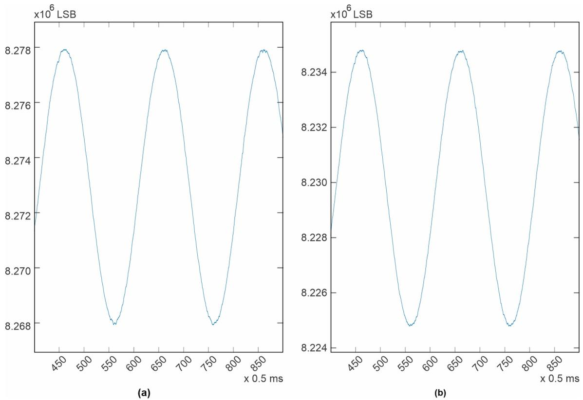
**Figure 6.** Test tone, 1 mV p-p sine wave, 10 Hz, sampling rate 2 kHz. (a) LA electrode; (b) V3 electrode.
