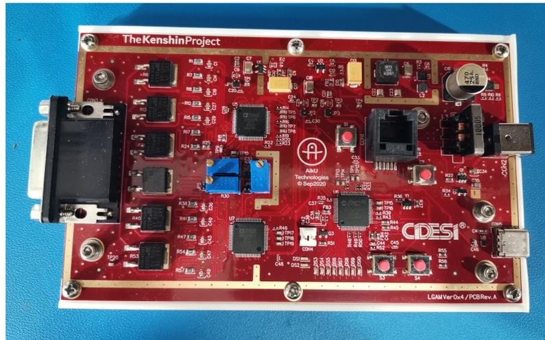
Figure 1. The Kenshin Device PCB (printed circuit board).
