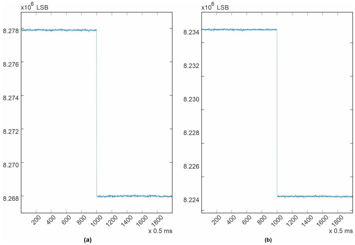
**Figure 5.** Test tone, 1mV square wave, 1 Hz, one cycle shown, sampling rate 2 kHz. (a) LA electrode; (b) V3 electrode.
