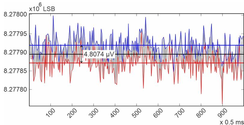
**Figure 9.** Illustration of the methodology for calculating the system’s noise. In blue, the peaks of the system’s noise and its average value. In red, the valleys of the system’s noise and its average value. In black, the average value of peaks and valleys together.
