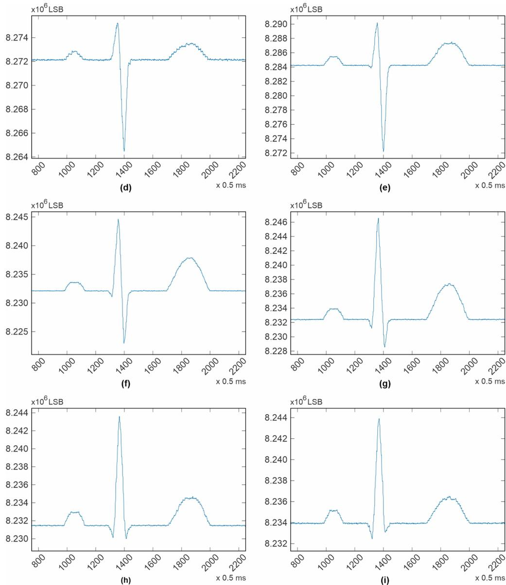
**Figure 8.** ECG signals from the FLUKE PS420 patient simulator: (a) LA electrode, (b) LL electrode, (c) RA electrode. (d) V1 electrode, (e) V2 electrode, (f) V3 electrode, (g) V4 electrode, (h) V5 electrode, and (i) V6 electrode.
