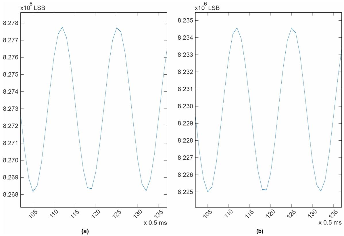
**Figure 7.** Test tone, 1 mV p-p sine wave, 150 Hz, sampling rate 2 kHz. (a) LA electrode; (b) V3 electrode.
