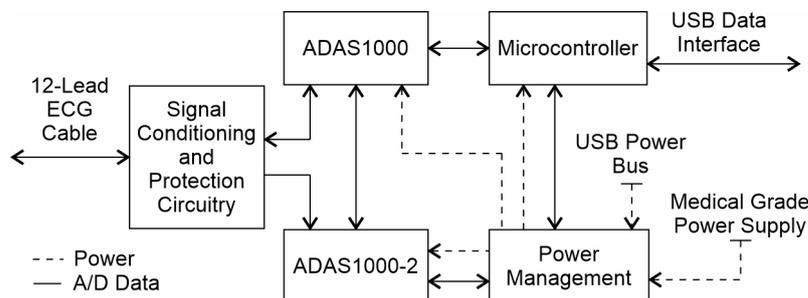
**Figure 4.** Functional block diagram of the Kenshin Device.
