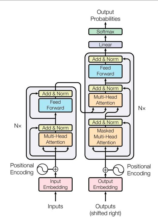
Figure 4. Transformer architecture [25].
