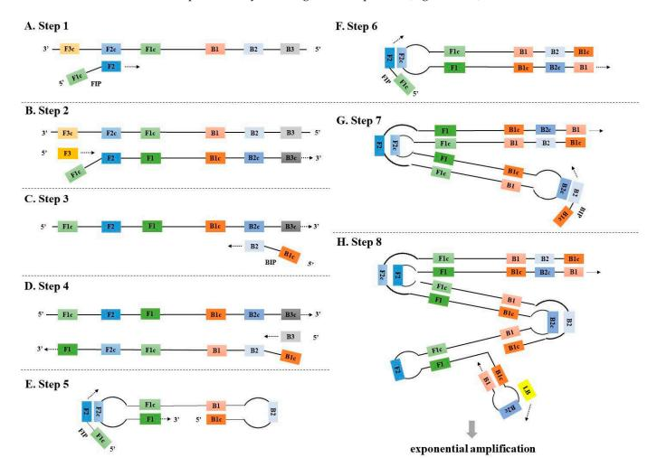
**Figure 1.** The principle of the traditional LAMP. F3 and B3: Forward and backward outer primers, respectively; FIP (F1c + F2) and BIP (B1c + B2): Forward and backward inner primers, respectively; LF and LB: Forward and backward loop primers, respectively.
