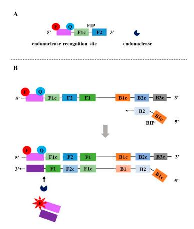
Figure 6. The principle of the MERT-LAMP. F: fluorophore; Q: quencher.
