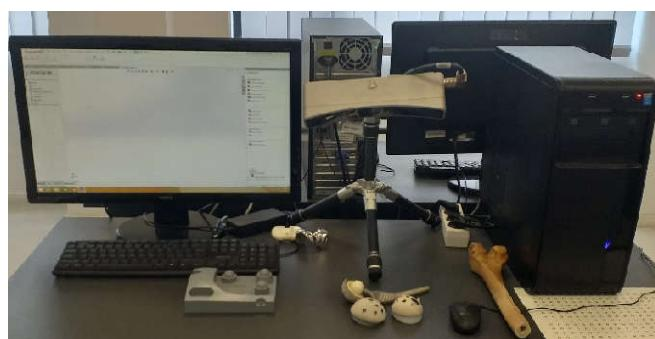
**Figure 17.** 3D Geomagic Capture Scanner.
