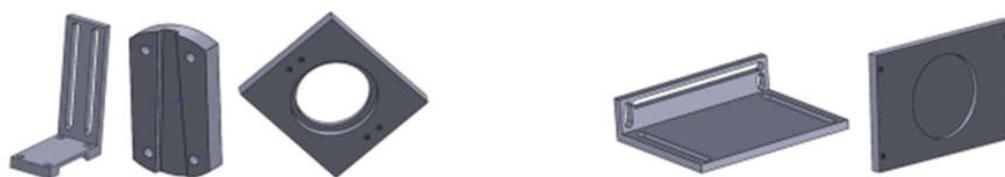
**Figure 15.** Virtual components of the fixing device.
