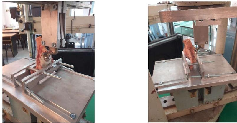
**Figure 18.** The prosthesis with titanium augment fixed on the EDZ20 machine.
