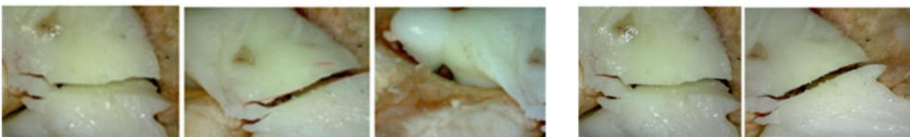
**Figure 20.** Micro fissures in the orthopaedic prosthesis analysed under the microscope.
