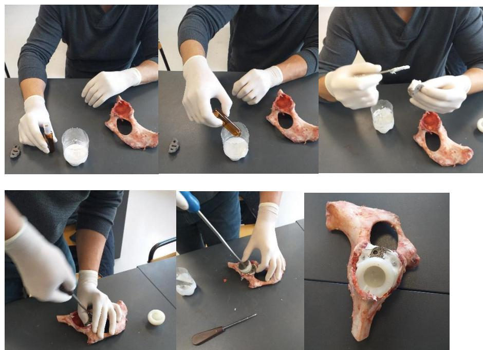
**Figure 5.** Steps for fixation of prosthesis elements using orthopaedic cement.
