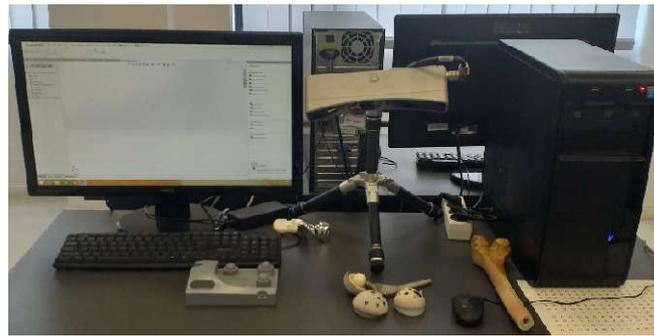
**Figure 17.** 3D Geomagic Capture Scanner.
