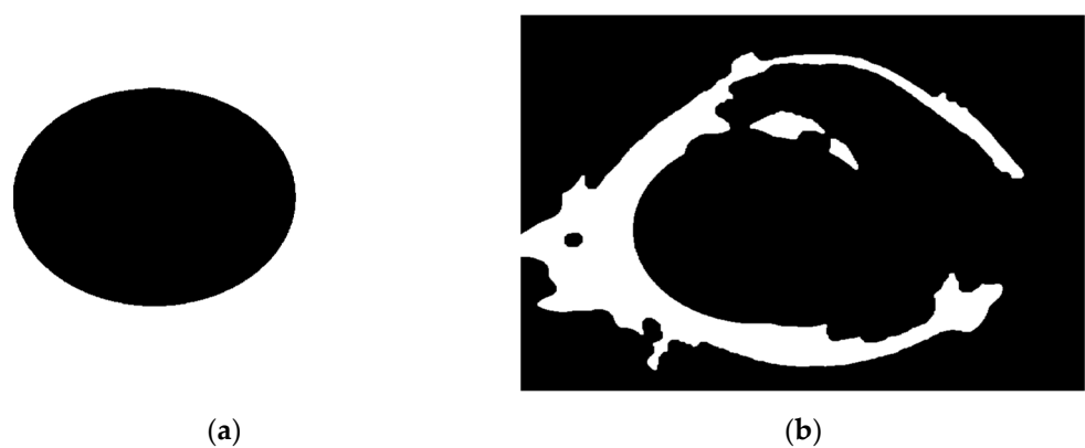
Figure 4. (a) The ellipse mask, (b) the binarized image of Figure 3, (b) after closing and masking with ellipse mask.
