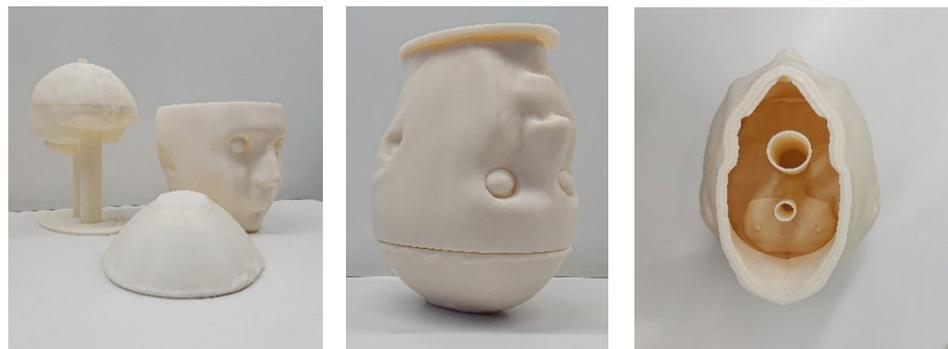
**Figure 3.** Upside-down configuration of the head phantom including the simple brain cavity.
