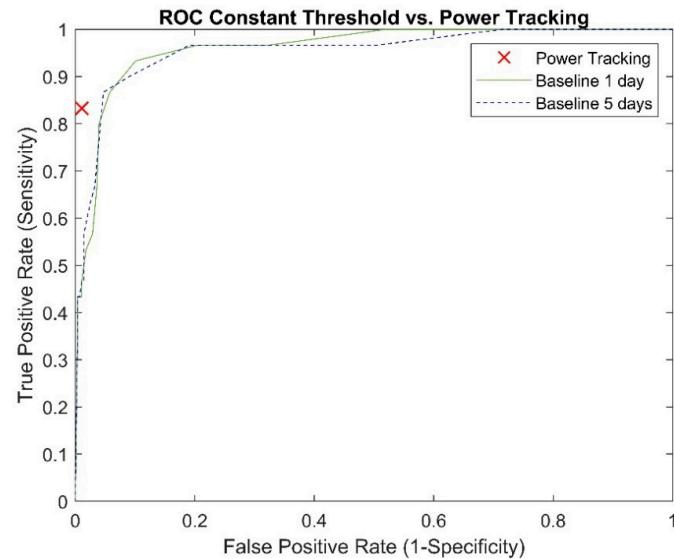
**Figure A1.** Receiver operating characteristic analysis of the power tracking algorithm, and with constant threshold (from 0.1 to 2.5 W) for a baseline of 1 and 5 days to determine pump power consumption baseline.
