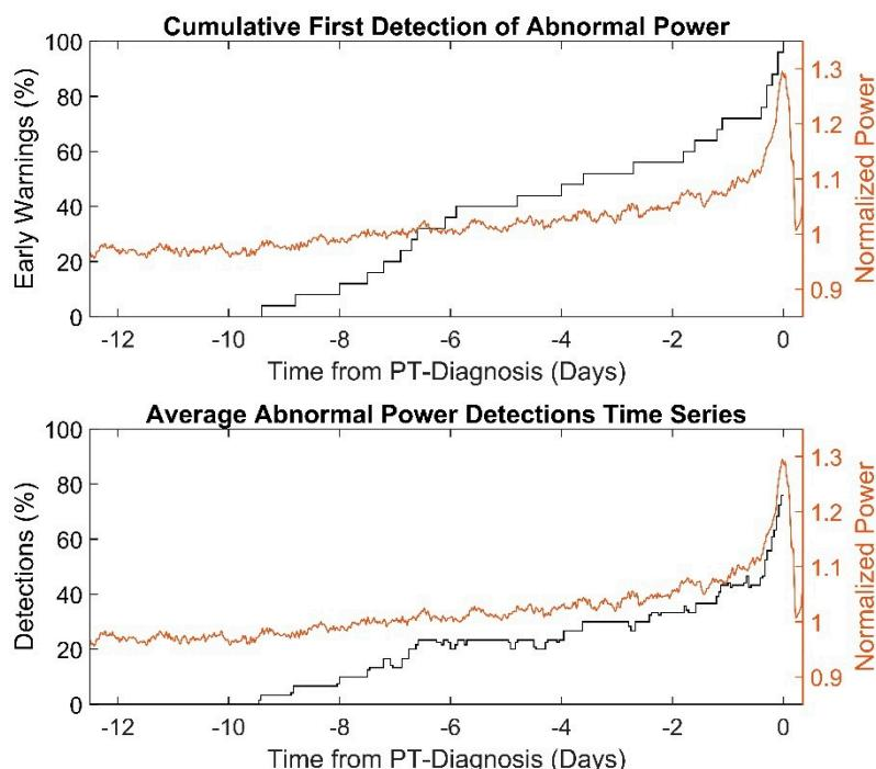
**Figure 2.** First detection of abnormal pump power cumulated across PT snapshots (top) and abnormal detections time series in the PT snapshots (bottom) with average normalized pump power signature (right ordinates).
