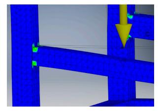
Figure 3. Stress simulation for the frame (von Mises stress).
