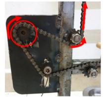
(c) Sprocket configuration on the motor bracket
