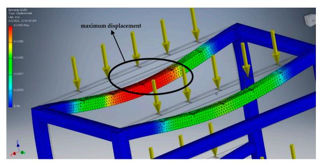
Figure 2. Stress simulation results for the frame (displacement).
