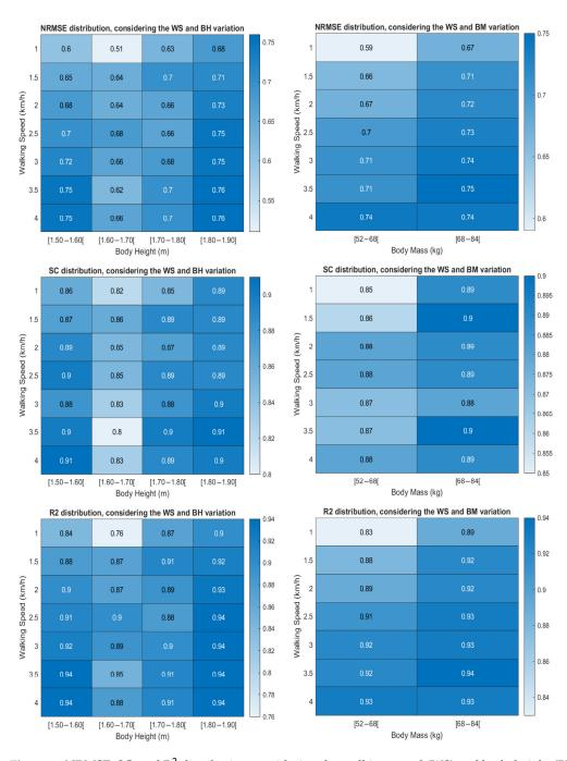
**Figure 5.** NRMSE, SC, and R<sup>2</sup> distribution considering the walking speed (WS) and body height (BH) variation (**left**), and the WS and body mass (BM) variation (**right**).
