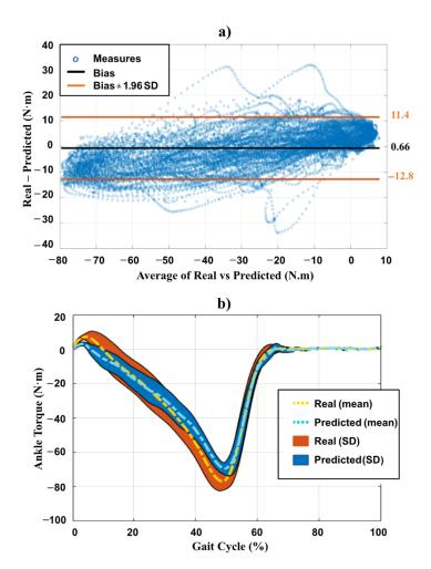
**Figure 4.** (a) Bland–Altman plot results; (b) Mean (dashed lines) and SD (filled area) of the real and CNN-based predicted ankle joint torque for the test dataset.
