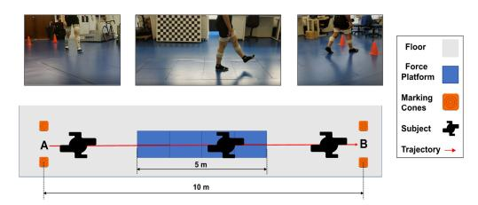
**Figure 2.** Data acquisition scenario, in which points A and B represent the beginning and the end positions of each trial, respectively.
