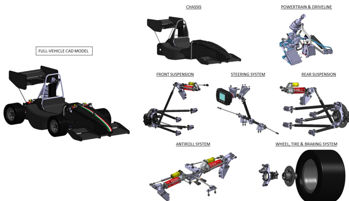
Figure 1. Subsystem integration leading to a full vehicle model—original CAD design.
