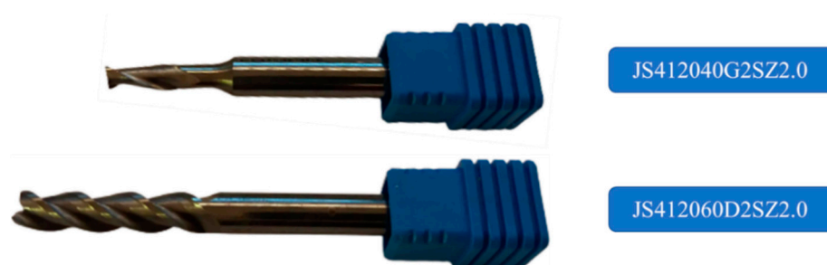
Figure 2. Images of the two different solid carbide end mills used for the experiments.
