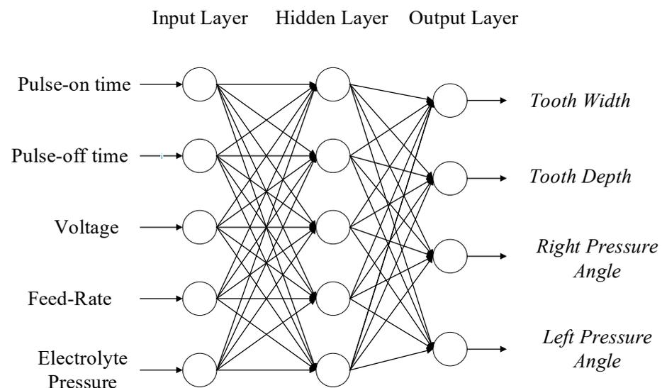
**Figure 4.** Neural network structure used for prediction of outputs.
