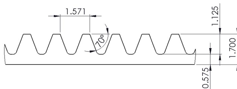
**Figure 3.** The desirable dimensions of the saw tooth profile ( $m = 0.5$ ). All dimensions are in millimeters (mm).
