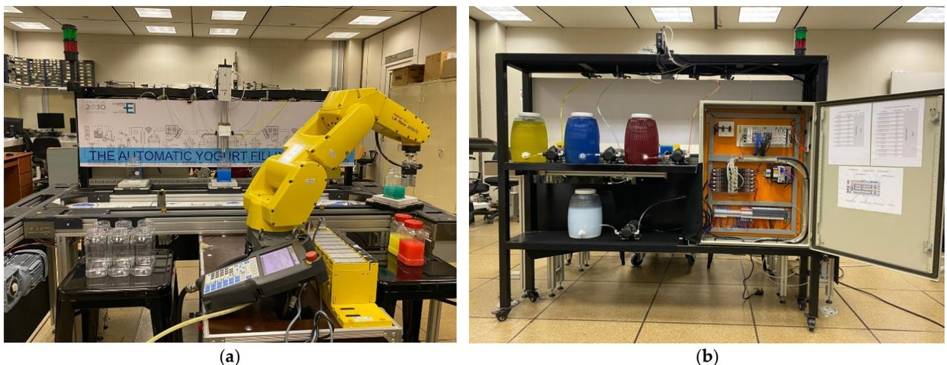
**Figure 5.** Designed smart yogurt filling machine and implementation: (a) main components of the proposed system at the front side, including robotic arm, conveyor belt, solenoid valves nozzle with three heads, proximity sensors, and cup/filling pneumatic actuators; (b) main components of the proposed system at the back side, including filling containers (plain yogurt and flavored), and electrical control panel with WAGO PFC controller.
