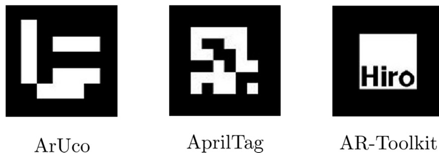
Figure 1. Examples of square fiducial markers.
