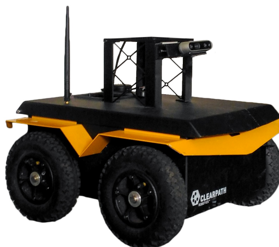
Figure 1. UGV Jackal from Clearpath Robotics endowed with an Intel RealSense D435i.
