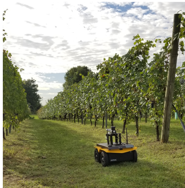
Figure 8. Jackal model robotic platform on the test site during the field experimentation.
