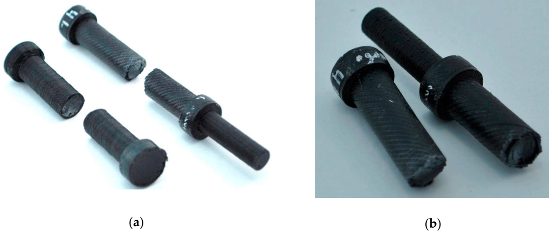
Figure 16. Cylindrical samples after testing: (a) standard 3D printing sample (left) and 4-layer 5D printing sample (right); (b) enlarged view of the fracture place.
