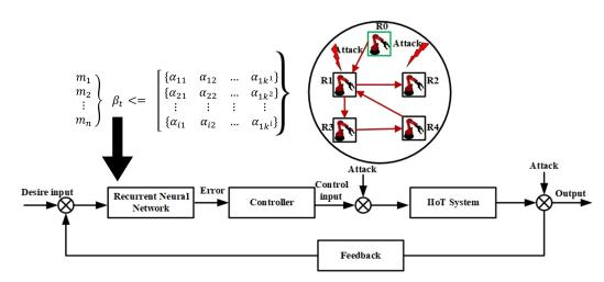
Figure 8. RNN- and SMC-based closed-loop feedback control mechanism for an IIoT system.
