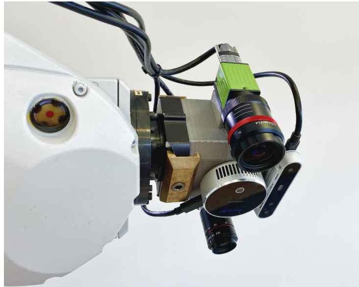
Figure 5. Different camera sensors were attached to the end-effector of an industrial robot.
