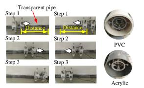
Figure 17. In-pipe robot prototype test of forward and reverse motion.
