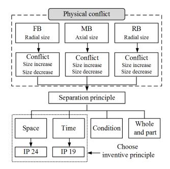
Figure 9. Physical conflict in the peristaltic in-pipe robot.
