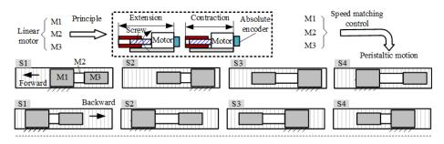
**Figure 2.** Traditional two-direction peristaltic robot driven by 3-motor structure (move forward and move backward).
