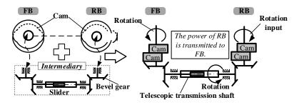
Figure 13. Intermediary—telescopic transmission shaft.
