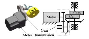
Figure 10. Motor-driven cam.
