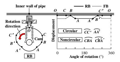
Figure 11. Periodic action of the cam.
