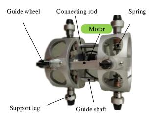
Figure 4. Novel in-pip robot prototype.
