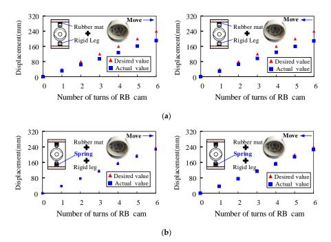
Figure 19. Walking test in PVC pipe: (a) test without spring; (b) test with spring.
