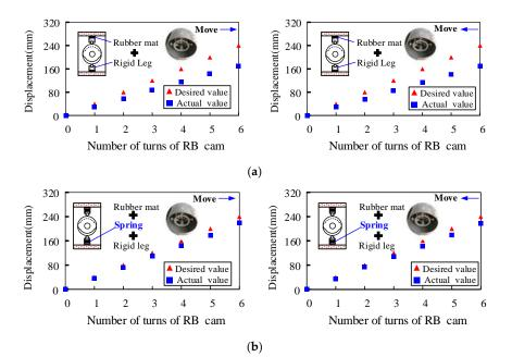
Figure 18. Walking test in acrylic pipe. (a) test without spring; (b) test with spring.
