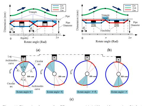
**Figure 16.** Dimension changes when RB cam rotates: (**a**) rigid leg without spring; (**b**) elastic leg with spring inside; (**c**) RB cam rotation status.
