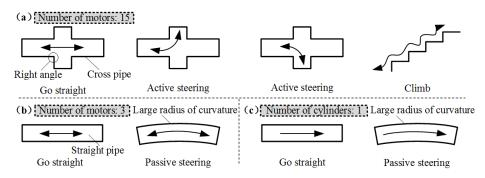
**Figure 1.** Move direction classification of peristaltic robots: (**a**) multi-direction, (**b**) two-direction, (**c**) one-direction.
