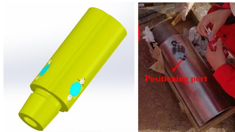
Figure 4. Structure and physical diagram of vibration measuring device.
