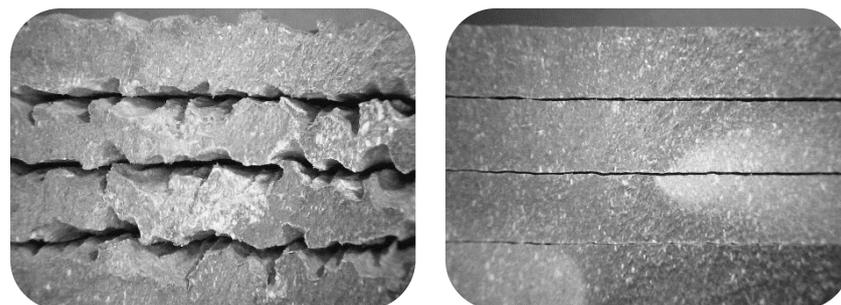
Figure 8. Cut at water jet outlet (left: Q1 set samples/right: Q5 set samples).
