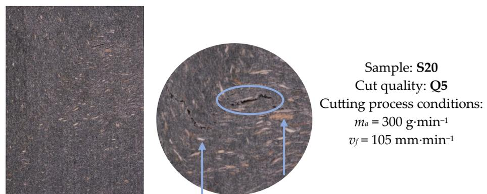
**Figure 9.** Significant cracks at the top of the profile cut by AWJ (arrows are pointing on natural reinforcement with different fractions and colours).
