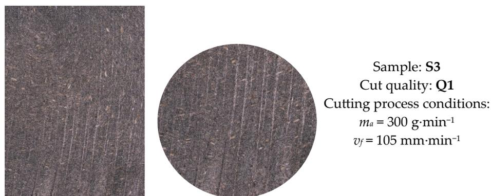
**Figure 10.** Pronounced furrows (tracks) left by AWJ in the final area of the cut.
