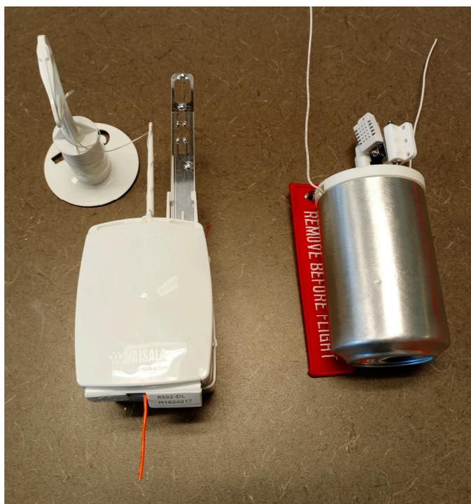
**Figure 4.** Vaisala RS92-DL radiosonde (Left) compared to a meteorological CanSat (Right).
