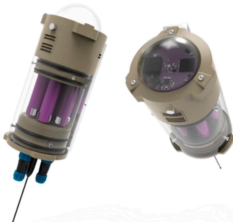
**Figure 2.** Rendering of Low-cost Air Quality Monitoring CanSat as seen from two angles, licensed under Creative Commons by [20].
