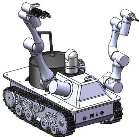
Figure 2. The schematic of the explosive ordnance disposal robot.
