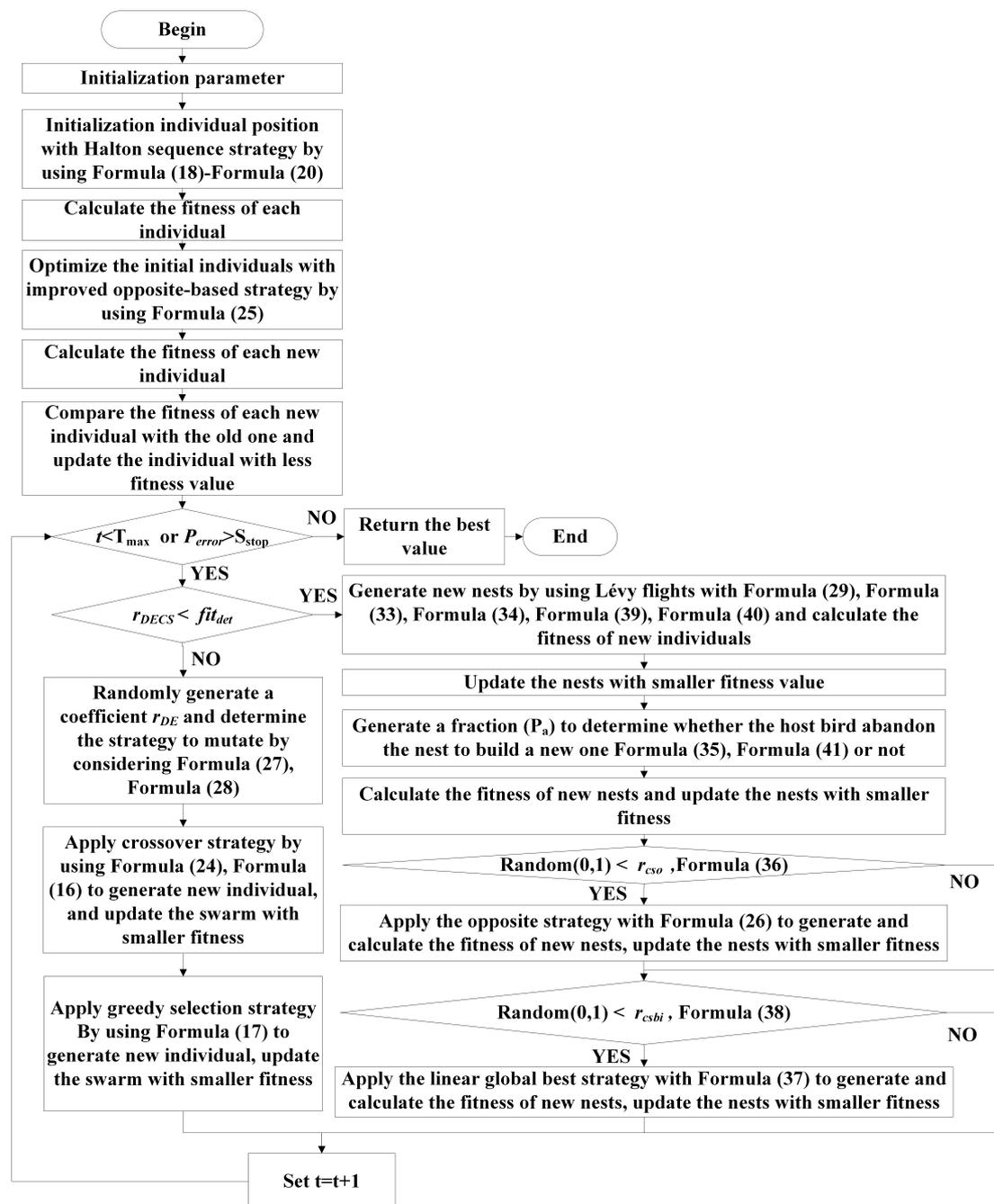
Figure 1. The schematic diagram of BODE-CS algorithm.
