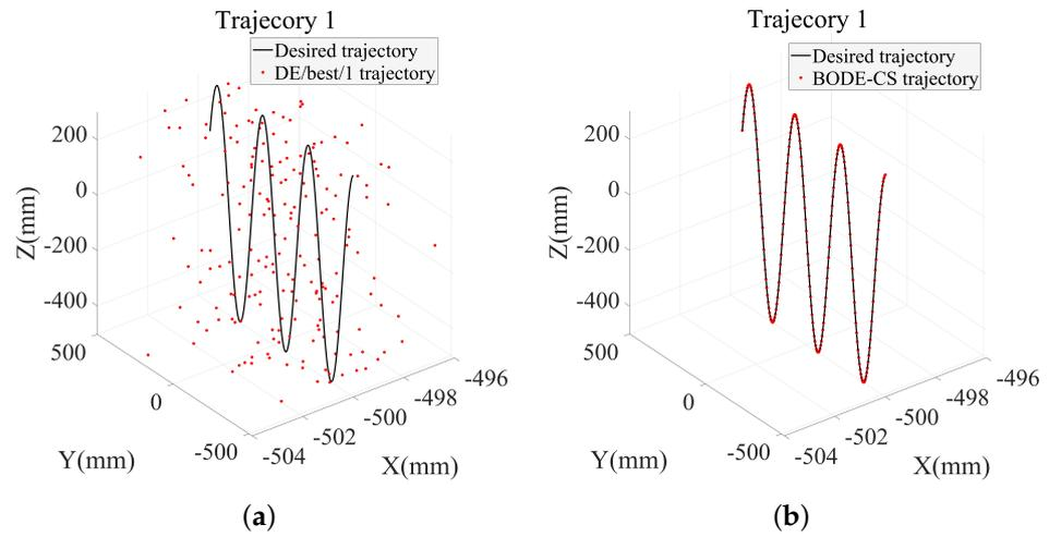
**Figure 17.** Trajectory 1 tracking results based on BODE-CS algorithm and DE/best/1 algorithm. (a) DE/best/1 algorithm. (b) BODE-CS algorithm.
