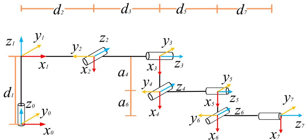
Figure 11. The coordinate system of Baxter’s manipulator using modified D–H method.
