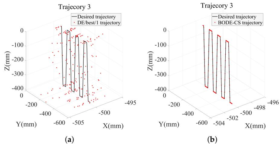
**Figure 19.** Trajectory 3 tracking results based on BODE-CS algorithm and DE/best/1 algorithm. (a) DE/best/1 algorithm. (b) BODE-CS algorithm.
