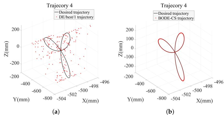
**Figure 20.** Trajectory 4 tracking results based on BODE-CS algorithm and DE/best/1 algorithm. (a) DE/best/1 algorithm. (b) BODE-CS algorithm.
