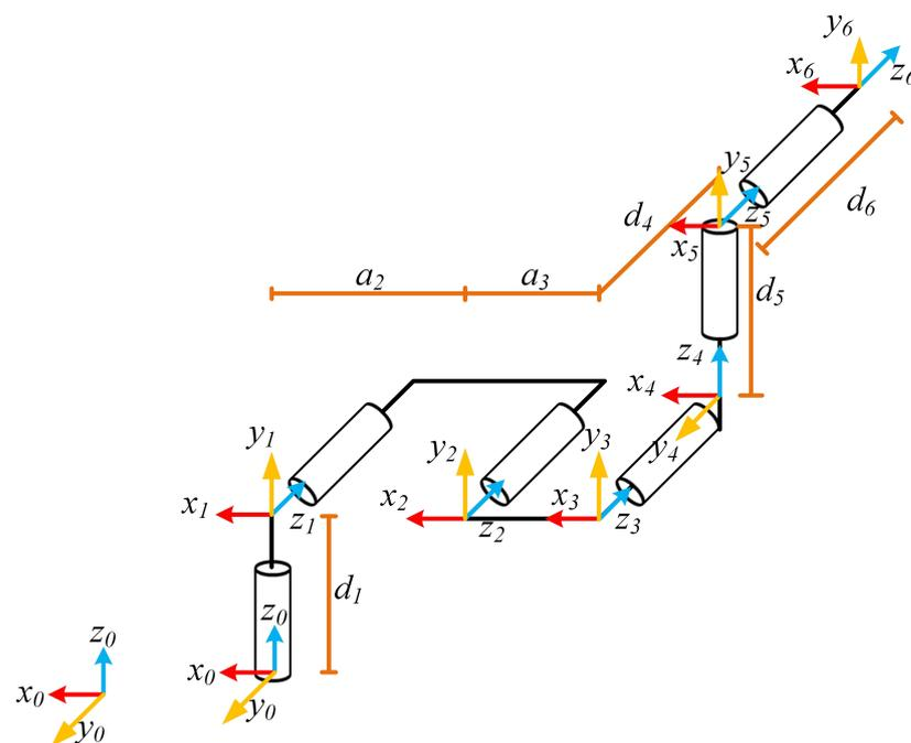
Figure 4. The configuration of the main manipulator using standard D-H method.
