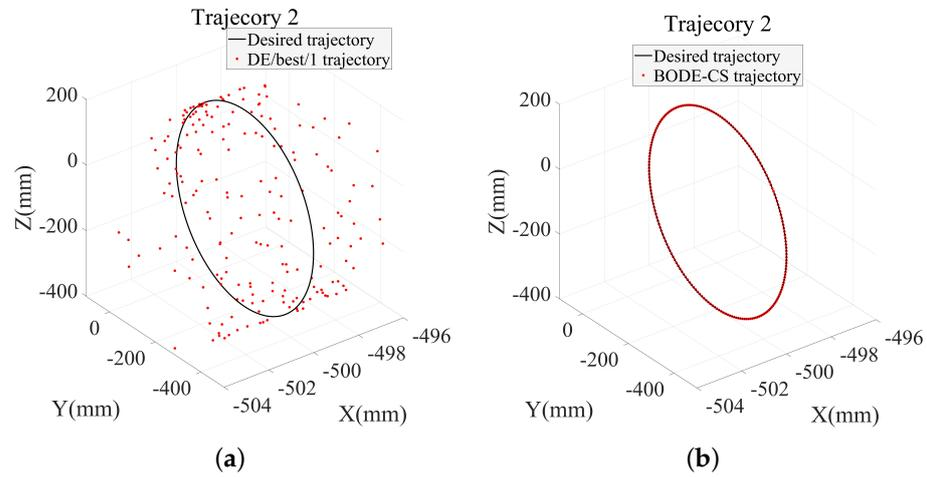
**Figure 18.** Trajectory 2 tracking results based on BODE-CS algorithm and DE/best/1 algorithm. (a) DE/best/1 algorithm. (b) BODE-CS algorithm.
