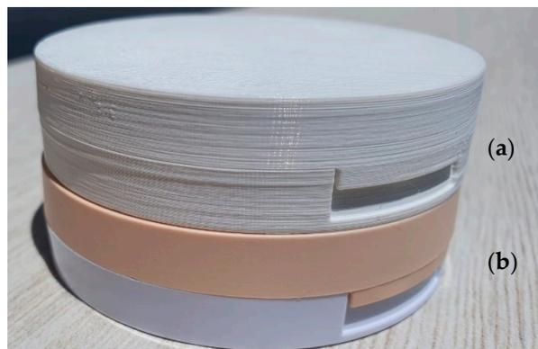
**Figure 5.** Surface finish comparison of (a) FFF and (b) IM compact.
