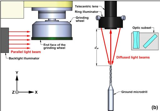
**Figure 6.** Illustrations of the working principles of the machine vision module: (a) the application for positioning the drilltip; (b) the application for measuring the CSGPs.
