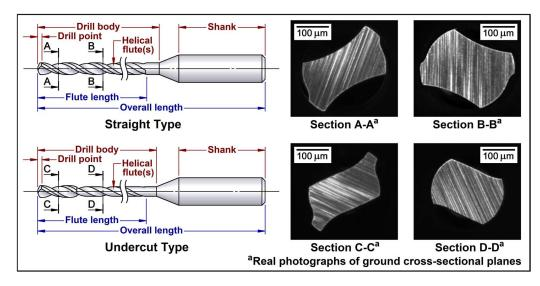
Figure 1. Illustrations and ground cross-sections of ST and UC type microdrills.
