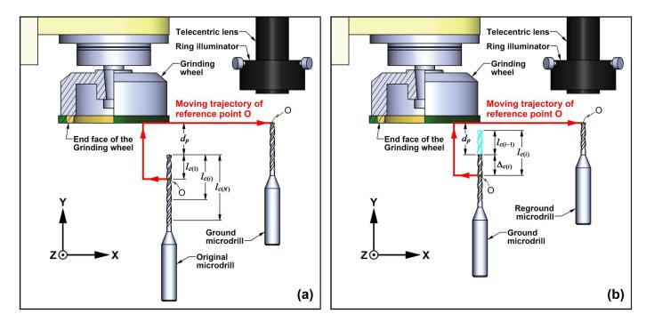
**Figure 11.** Schematic diagrams of the GO sub-process: (a) grinding off an original microdrill; (b) regrinding off a ground microdrill.
