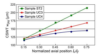
Figure 17. Measured values and fitted curves of the CSWTs of certain microdrill samples.
