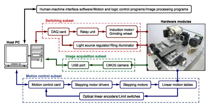
Figure 7. Functional block diagram of the improved automation system.
