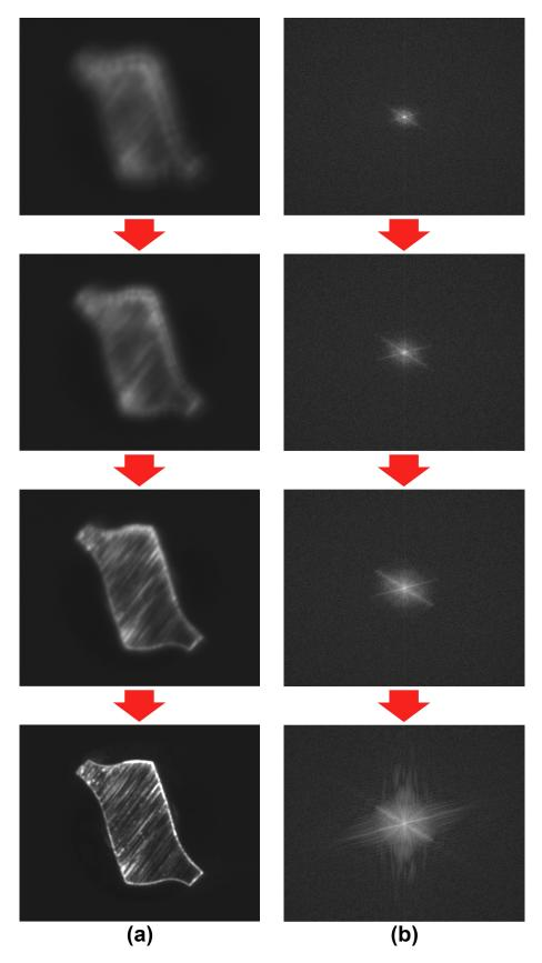
**Figure 12.** Illustration of the AF sub-process: (a) axial-viewed images captured from an unfocused condition to a clearly focused condition; (b) the corresponding centered Fourier spectra.
