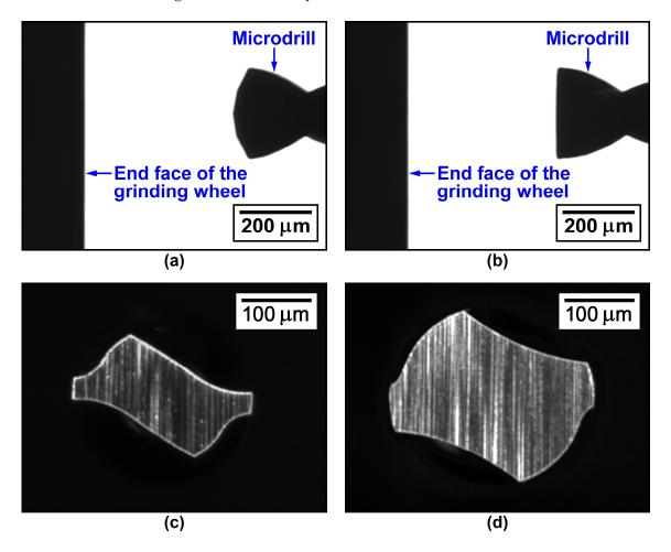
**Figure 8.** Digital images captured by the machine vision module: (a) a side-viewed image of an original microdrill sample; (b) another side-viewed image of a ground microdrill sample; (c) an axial-viewed image of a ground cross-section.
