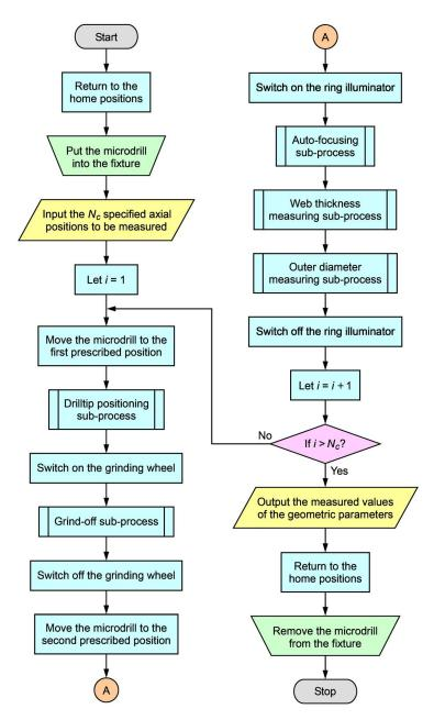
Figure 9. Main flowchart of the established AMP.
