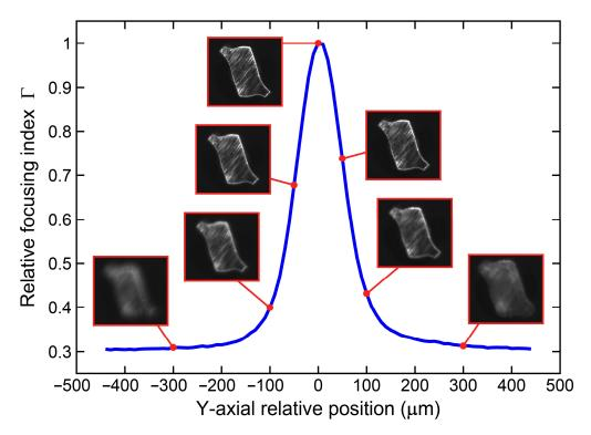
**Figure 13.** Illustrative example of the variation curve of the relative focusing index  $\Gamma$  with respect to the Y-axial relative position.
