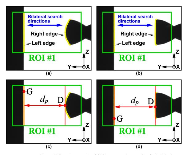
**Figure 10.** Illustrative examples of the image processing procedure for the DP sub-process: (a) edge detection for a side-viewed image; (b) edge detection for another side-viewed image; (c) measuring the positioning distance between the drilltip and the GWEF; (d) measuring the positioning distance between a certain ground cross-section and the GWEF.
