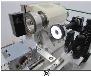
**Figure 5.** Closeup views of the machine vision module under its actual usage conditions: (a) the application for positioning the drilltip; (b) the application for measuring the CSGPs.
