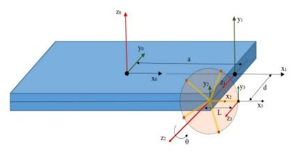
Figure 7. Robot kinematics image.
