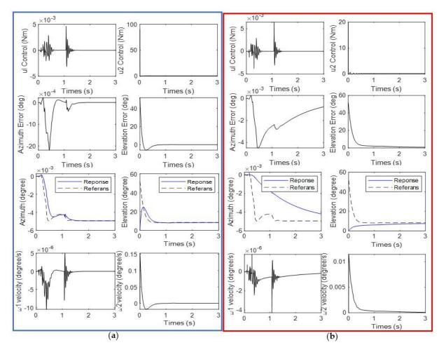
graphs show that both controllers perform well at the tracking azimuth angle, but the SMC controller outperforms the PID controller when it comes to controlling the elevation angle.
