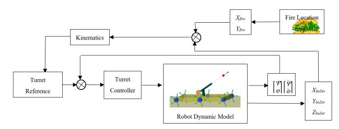
**Figure 12.** Schematic representation of firefighting robot SimMechanics Simscape multibody simulation model.
