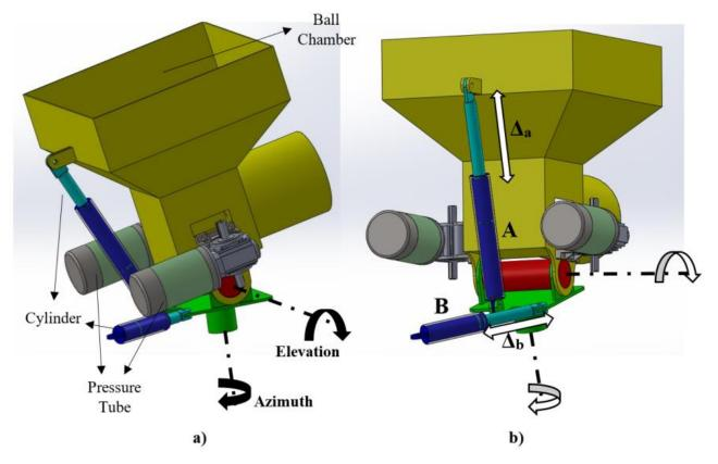
Figure 6. (a) Components used in the shooting turret (b) Shooting turret mechanism.
