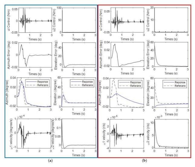
**Figure 16.** Control signals, error values, trajectory and velocity of Turret System elevation and azimuth motor with (**a**) SMC (**b**) PID controllers for Scenario 2.
