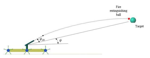
Figure 11. The oblique shot movement of the fire-extinguishing ball leaving the barrel.
