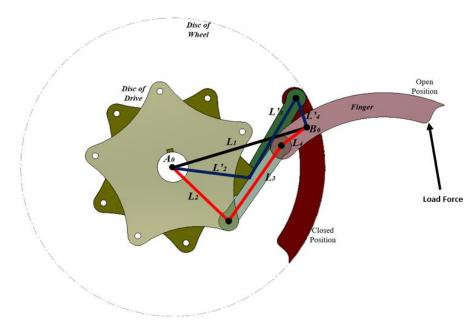
Figure 5. Four-bar mechanism for the movement of the fingers.
