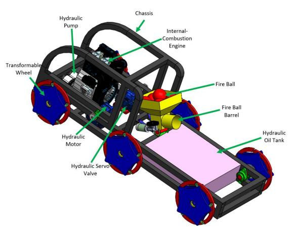
Figure 2. CAD views of designed Fire Fighting Robot with Fire Extinguishing Ball Shooting System.
