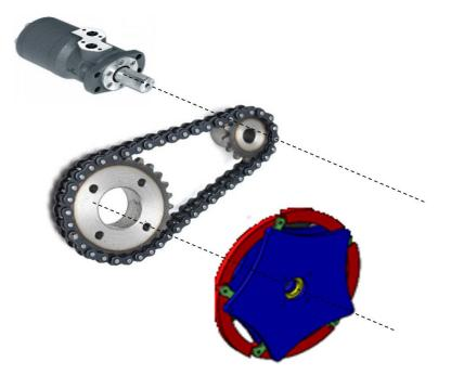
Figure 3. Wheel drive system of hydraulic motor with a gear-chain system.
