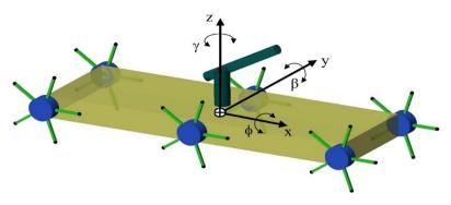
Figure 8. Euler angles of the robot body center.
