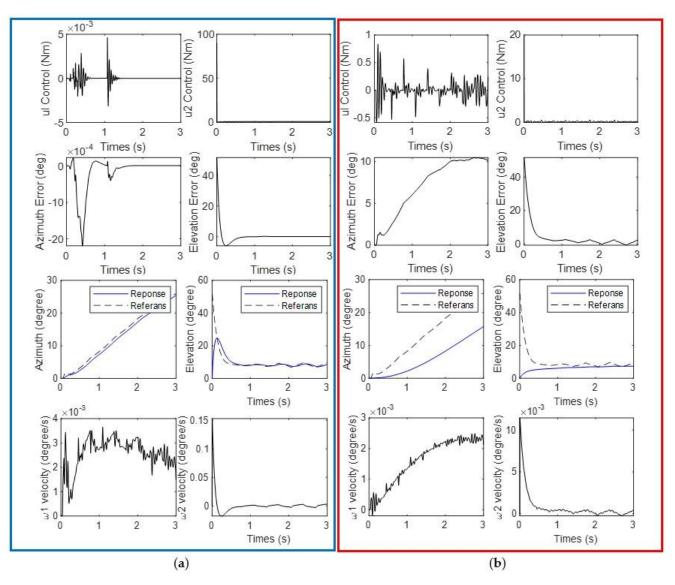
**Figure 18.** Control signals, error values, trajectory and velocity of Turret System elevation and azimuth motor with (**a**) SMC (**b**) PID controllers for Scenario 3.
