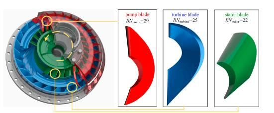
Figure 1. An anatomy diagram of a hydraulic torque converter.
