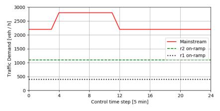
**Figure 4.** Traffic demand on the mainstream and on-ramps during simulation. Reprinted with permission from Ref. [8]. 2023, Filip Vrbanić.
