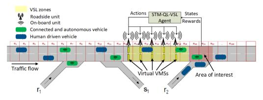
Figure 3. Configuration of the simulation model and VSL controllers. Adapted with permission from Refs. [5,7,8]. 2023, Filip Vrbanić.
