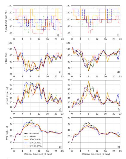
Figure 5. Obtained speed limits, speeds, densities, and TTS for scenario 1 (a,c,e,g) and scenario 2 (b,d,f,h).
