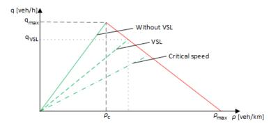
Figure 1. Speed limit effect on the fundamental diagram [6].
