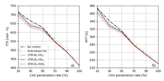
Figure 6. Change of TTT (a) and MTT (b) for different CAV penetration rates.
