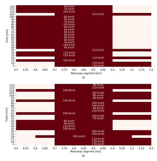
Figure 7. Obtained speed limit zone positions and computed speed limits for scenario 1 (a) and scenario 2 (b).
