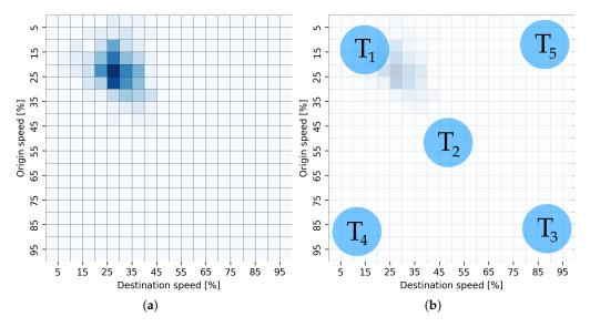
**Figure 2.** Examples of STMs representing congested traffic flow (**a**) and characteristic positions at STM (**b**).
