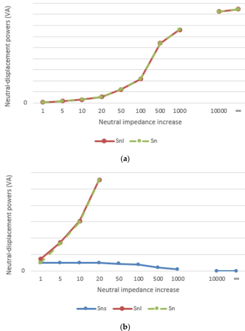
**Figure 2.** Typical increase of the the neutral-displacement powers during the breakage process of the neutral conductor in a three-phase system: (a) variation of  $S_n$  and  $S_{nl}$ ; (b) variation of  $S_{ns}$  in the same system, and detail of  $S_n$  and  $S_{nl}$ .
