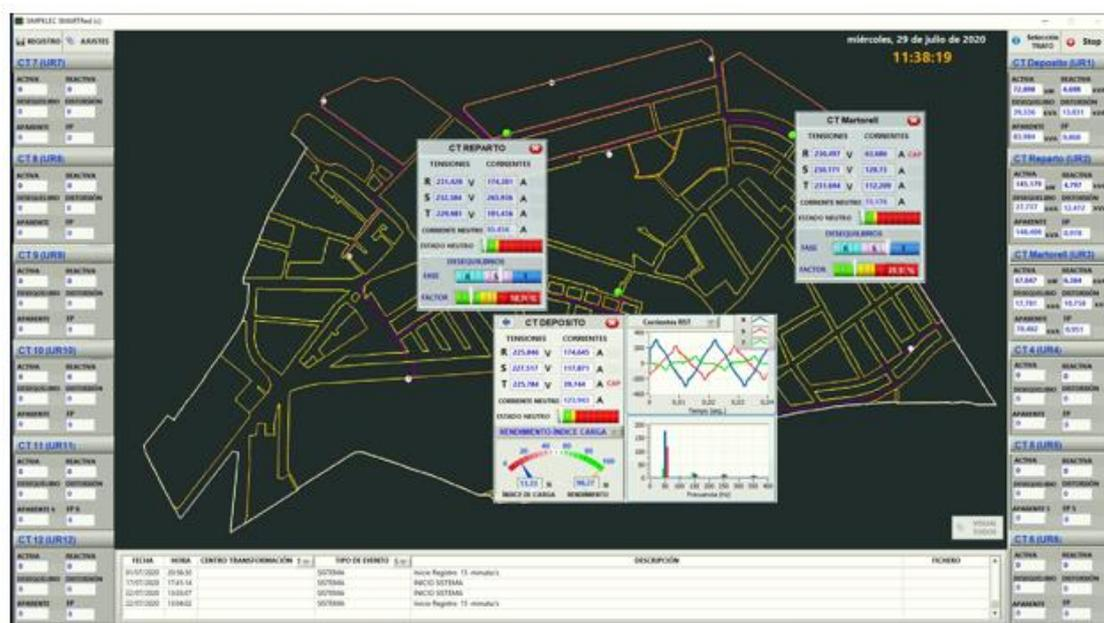
**Figure 5.** Main screen of the SIMPELEC-SMARTRed software, with representation of three monitored transformation houses (green points in the map of Vinales distribution network), and secondary screens showing parameters of these transformation houses.
