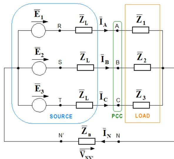
**Figure 1.** Three-phase four-wire wye-configured power system.
