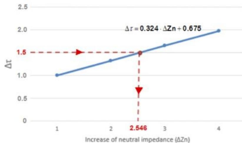
**Figure 3.** Growth pattern of the parameter  $\Delta\tau$  as a function of  $\Delta Z_n$  in the PCC of a distribution network, with a line of 300 mm<sup>2</sup> section and 16 m long (coefficients  $A = 0.324$  and  $B = 0.675$ ), and an example of determination of  $\Delta Z_n$  knowing the measured value of  $\Delta\tau = 1.5$ .
