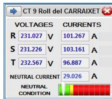
Figure 6. SIMPELEC-SMARTRed screen for monitoring the neutral conductor condition among other CT9 quantities. (It is noted the cursor is placed over the green zone).
