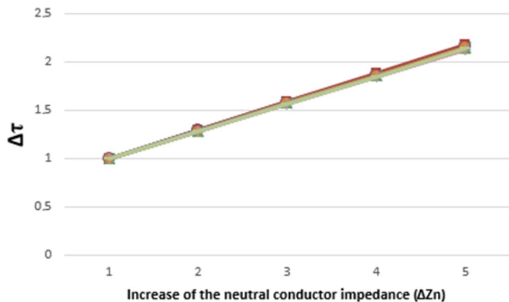
**Figure 8.** Growth lines of  $\Delta\tau$  as a function of the neutral conductor impedance increment ( $\Delta Z_n$ ) expressed in Table 11 for the different analyzed loads and regulation voltages.
