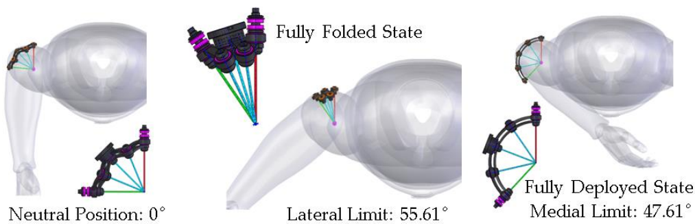
Figure 6. Wearing demonstration of the neutral, lateral limit, and medial limit state of the prototype development.
