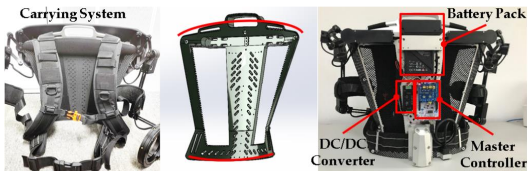
Figure 16. The carrying system and the electrical system installed on two sides of the back frame.
