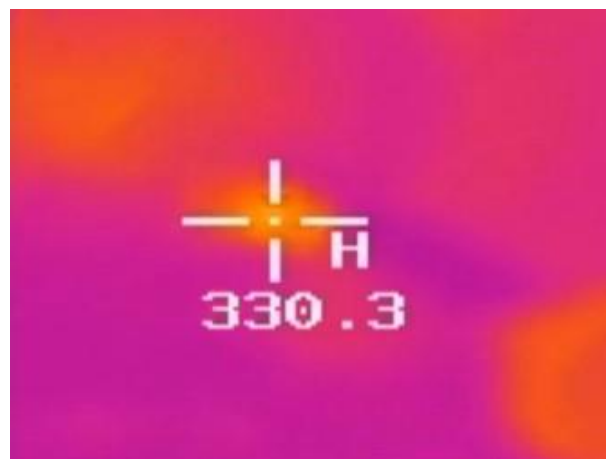
Figure 4. Cutting temperature thermal imaging.
