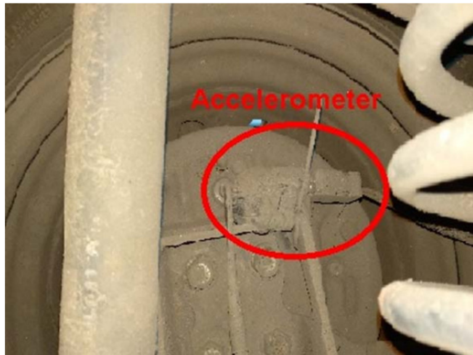
Figure 3. MEMS Accelerometer mounted on the test vehicle's rear axle.
