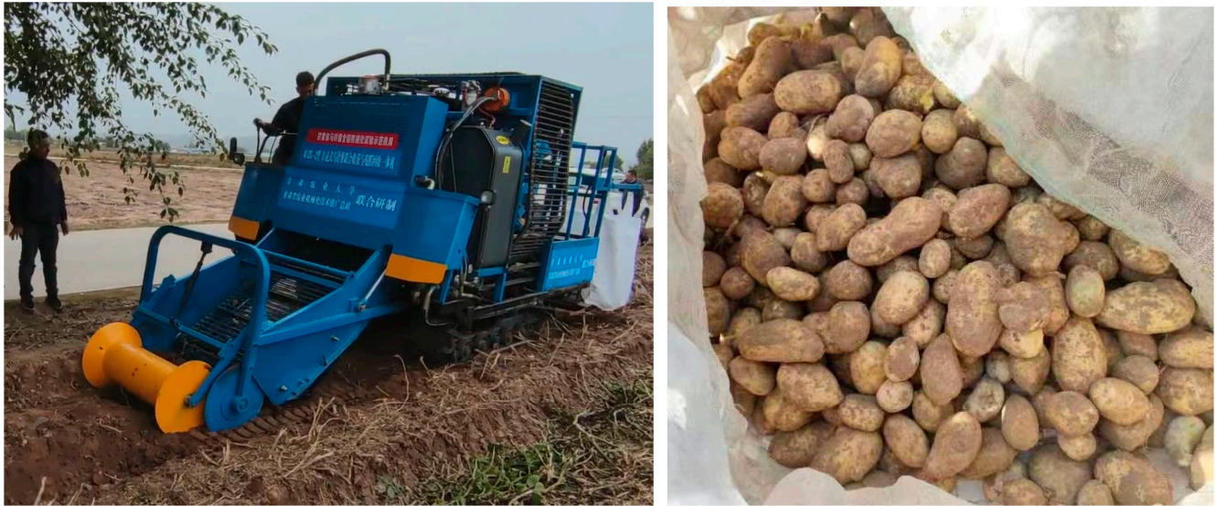
Figure 16. Field test showing the digging and lifting device of the self-propelled machine for combined potato harvesting and residual plastic film retrieval and a bag of harvested potatoes.
