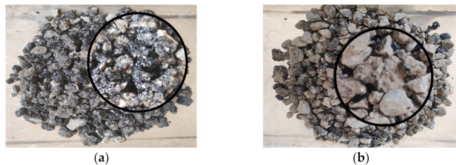
Figure 11. Surface morphology of coarse aggregates before and after treatment. (a) Surface color of coarse aggregates before treatment; (b) surface color of coarse aggregates after treatment.
