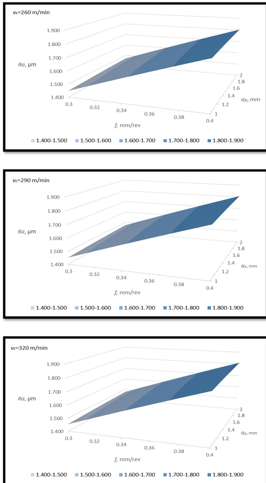
**Figure 5.** Achievable roughness parameter  $Ra$  when turning martensitic stainless steel X20Cr13 under MQL + vortex conditions for cutting speed ( $v_c$ ) = 260, 290 and 320 m/min: ( $f$ ) feed rate, ( $a_p$ ) depth of cut.
