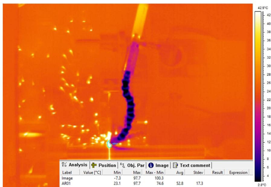
Figure 11. Temperatures in the cutting zone: MQL + vortex tube condition.
