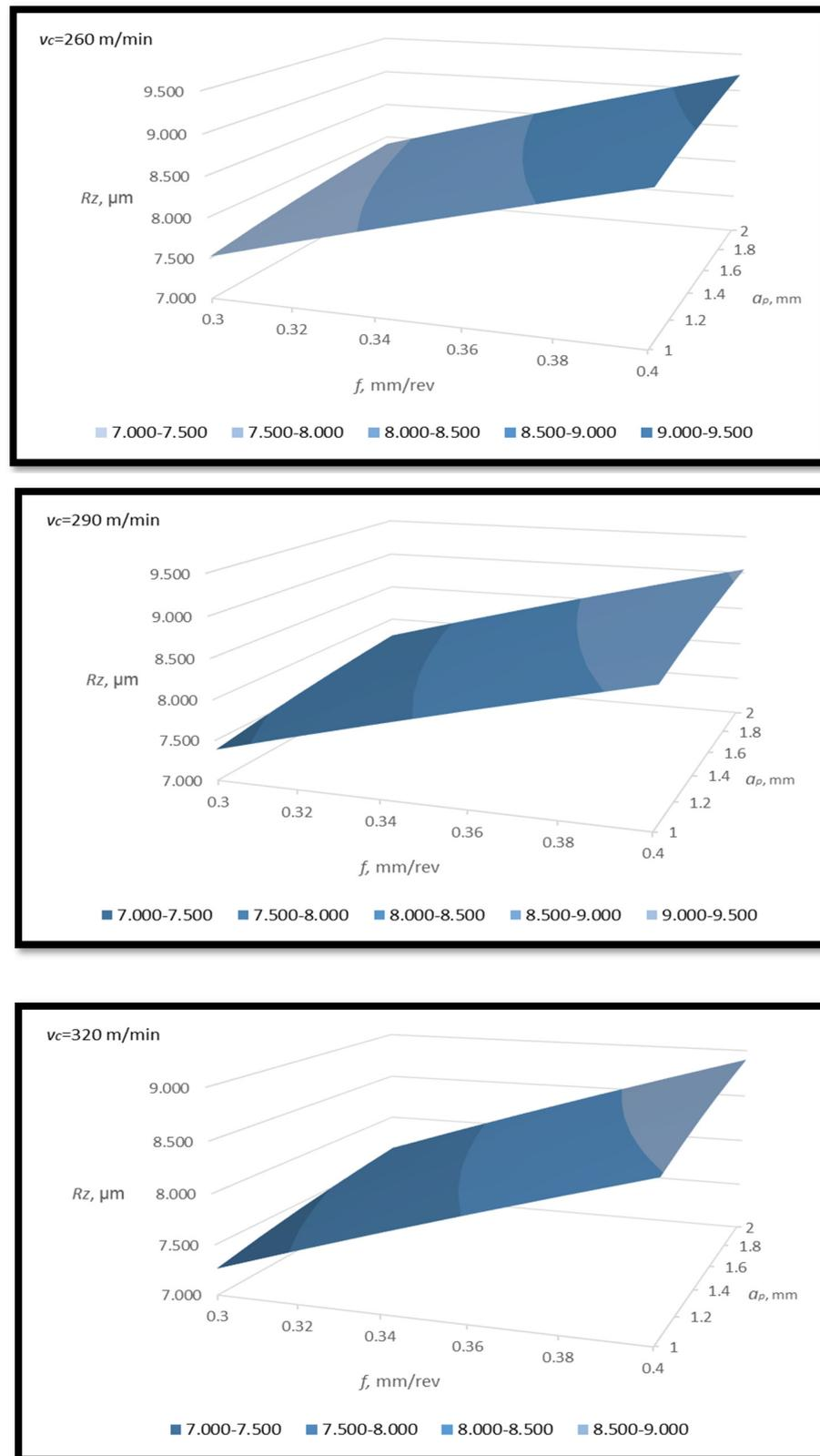
**Figure 7.** Achievable roughness parameter  $R_z$  when turning martensitic stainless steel X20Cr13 under MQL + vortex conditions for cutting speed ( $v_c$ ) = 260, 290 and 320 m/min: ( $f$ ) feed rate, ( $a_p$ ) depth of cut.
