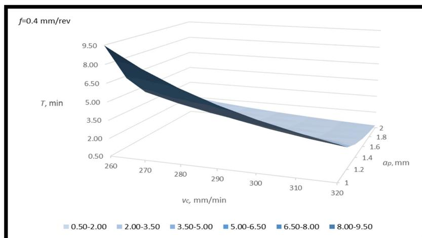
Figure 9. Achievable tool life ( $T$ ) when turning martensitic stainless steel X20Cr13 under.
