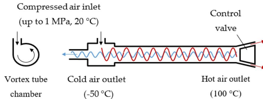
**Figure 2.** Counter-current flow vortex tube type.
