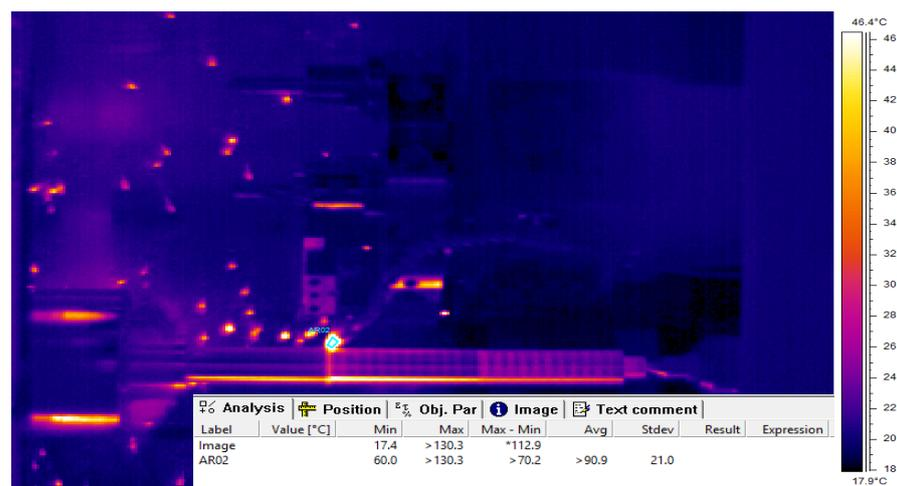
Figure 12. Temperatures in the cutting zone: MQL condition.
