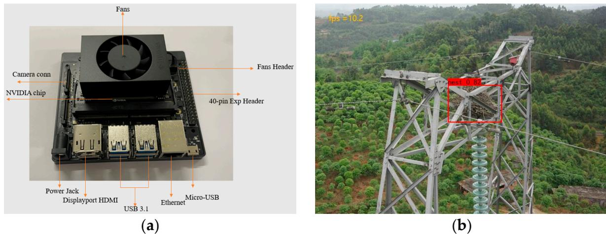
**Figure 14.** (a) Structure of Jetson Xavier NX; (b) real-time monitoring and collection results.
