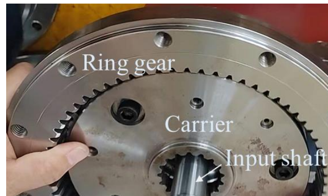
Figure 10. The photo of the planetary gear set assembly in the gearbox.
