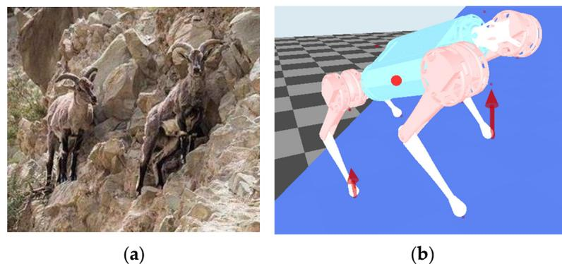
**Figure 1.** The uphill posture of blue sheep and the quadruped robot (under our adaptive algorithm). (a) Walking posture of blue sheep; (b) Walking posture under SAMPC.
