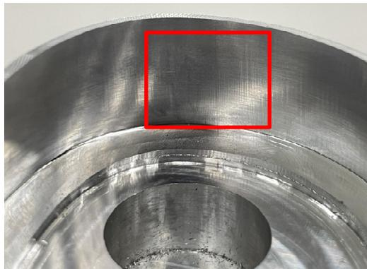
(c) roughness:  $Ra = 0.320 \mu\text{m}$
