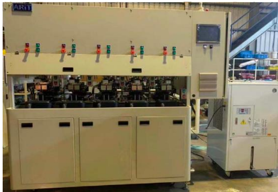
Figure 2. Vacuum degassing equipment.
