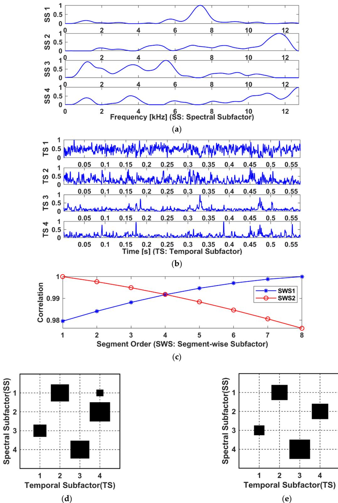
**Figure 7.** Factors of LRANTD: (a) the Spectral Factor, (b) the Temporal Factor, consisting of 4 temporal subfactors with kurtosis of 2.98, 4.1, 15.7, and 13.3, respectively, (c) the Segment-wise Factor with 2 subfactors, and (d) the Core Tensor represented via its frontal slice w.r.t. SWS1, and (e) that w.r.t. SWS2.
