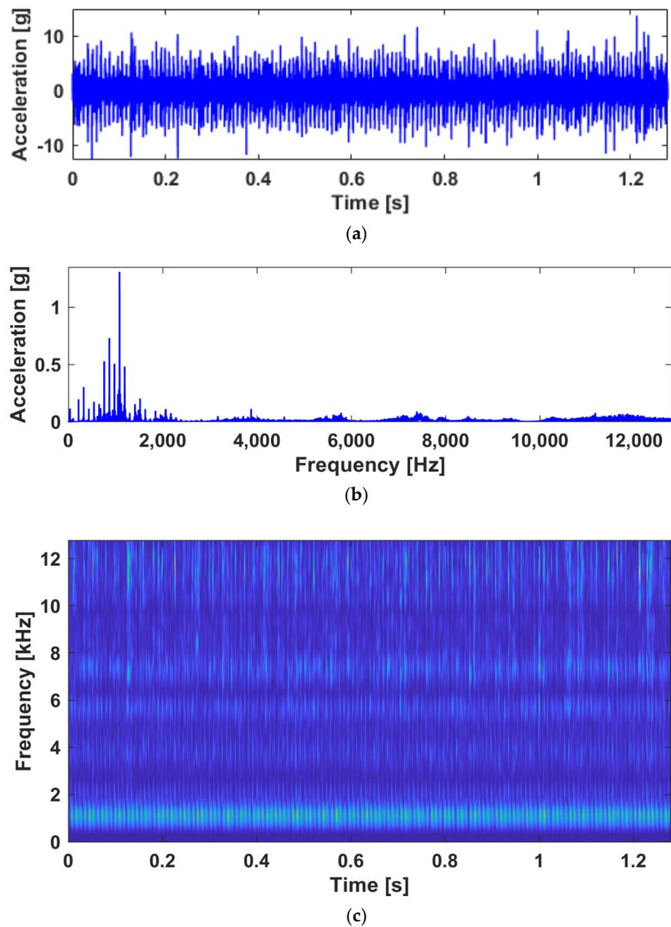
**Figure 12.** (a) The horizontal acceleration signal, (b) the amplitude spectrum, and (c) the corresponding STFT spectrogram in Case C.
