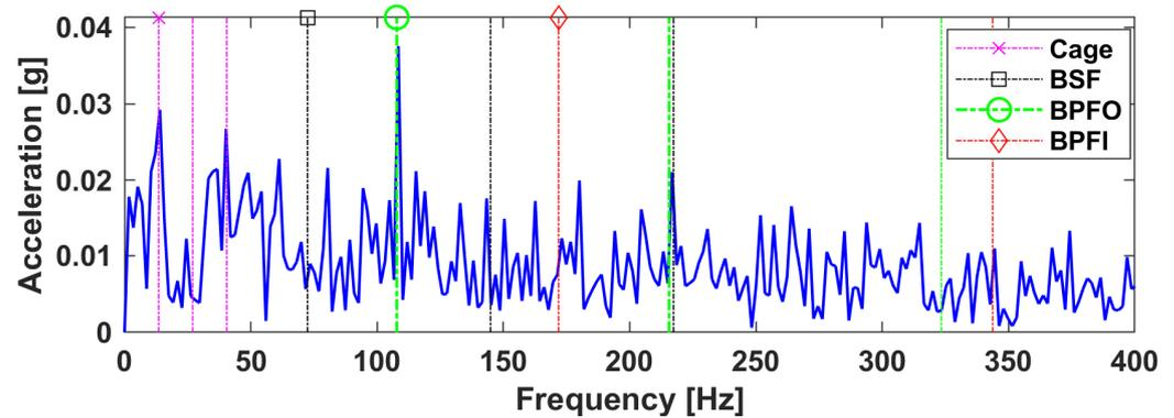
Figure 15. The amplitude spectrum attained by the LRANTD method in Case A (Proposed method).
