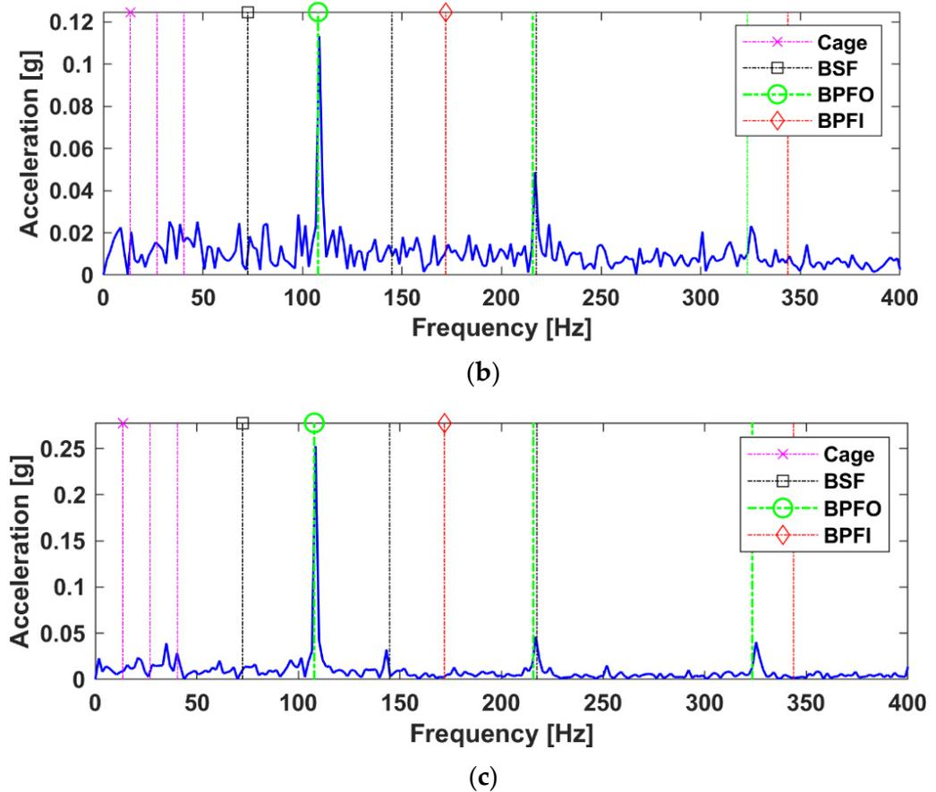
Figure 19. (a–c): The cross-spectra based on LRANTD fusion for Cases A to C. From Case A to Case C, the low-rank dimensions are, respectively, (3, 4, 2), (4, 4, 2), and (3, 3, 2).
