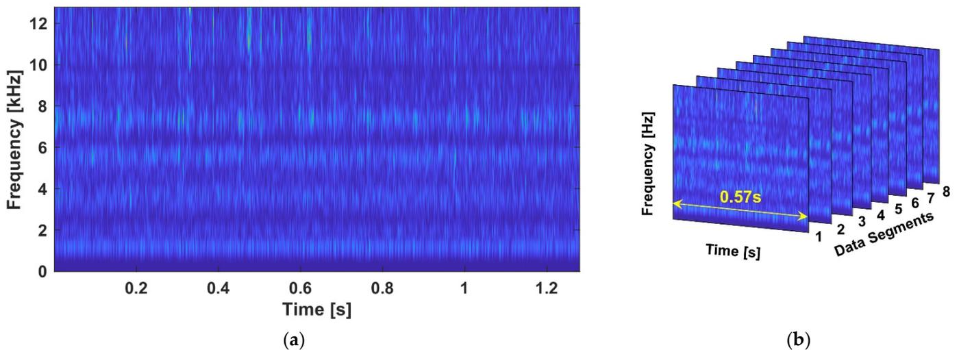
Figure 6. Time–frequency representations of the analysed data: (a) STFT spectrogram. (b) Time–frequency tensor reorganized from the spectrogram segments,  $\mathbf{y} \in \mathbb{R}^{256 \times 14640 \times 8}$ .
