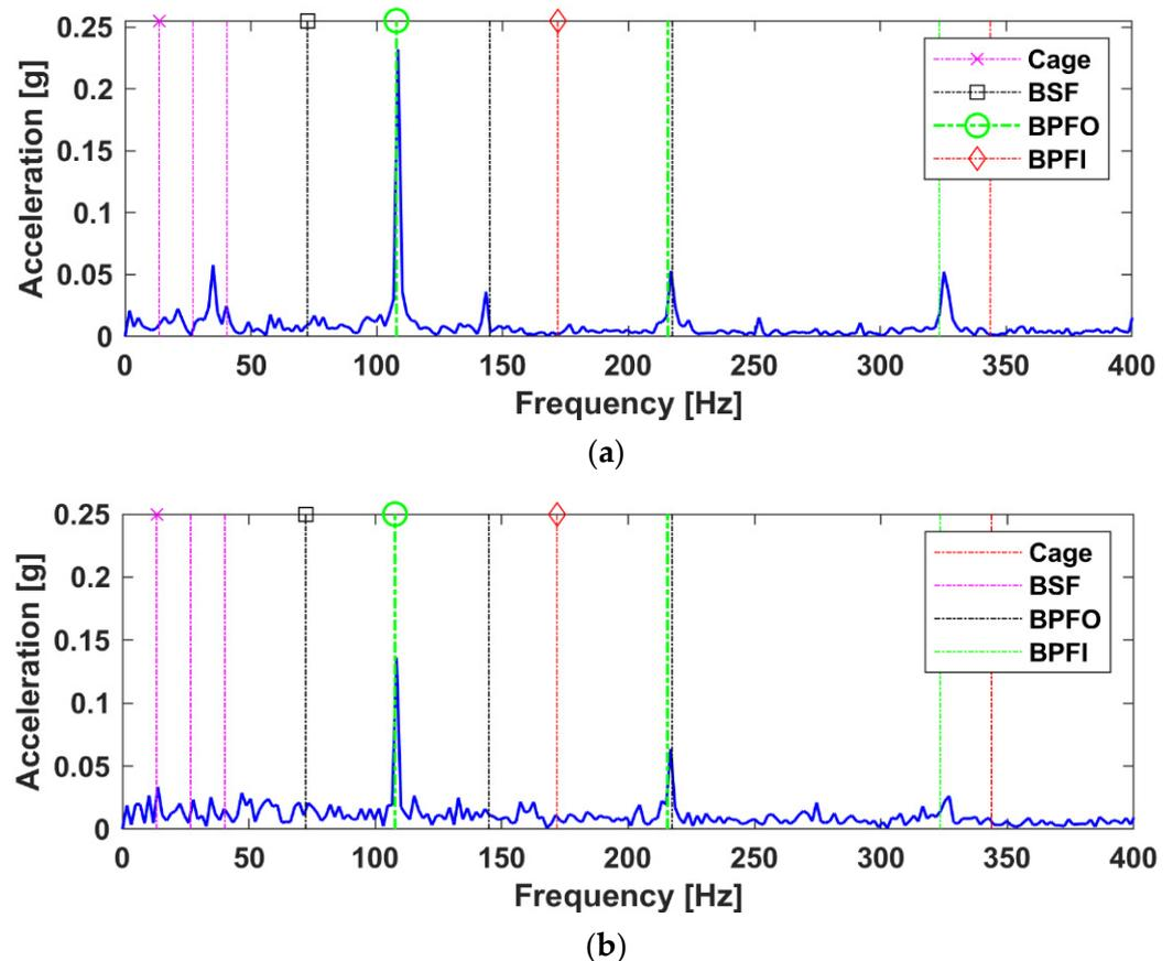
**Figure 14.** Case C results via LRANTD. (a) The amplitude spectrum of TS1 and (b) that of TS3.
