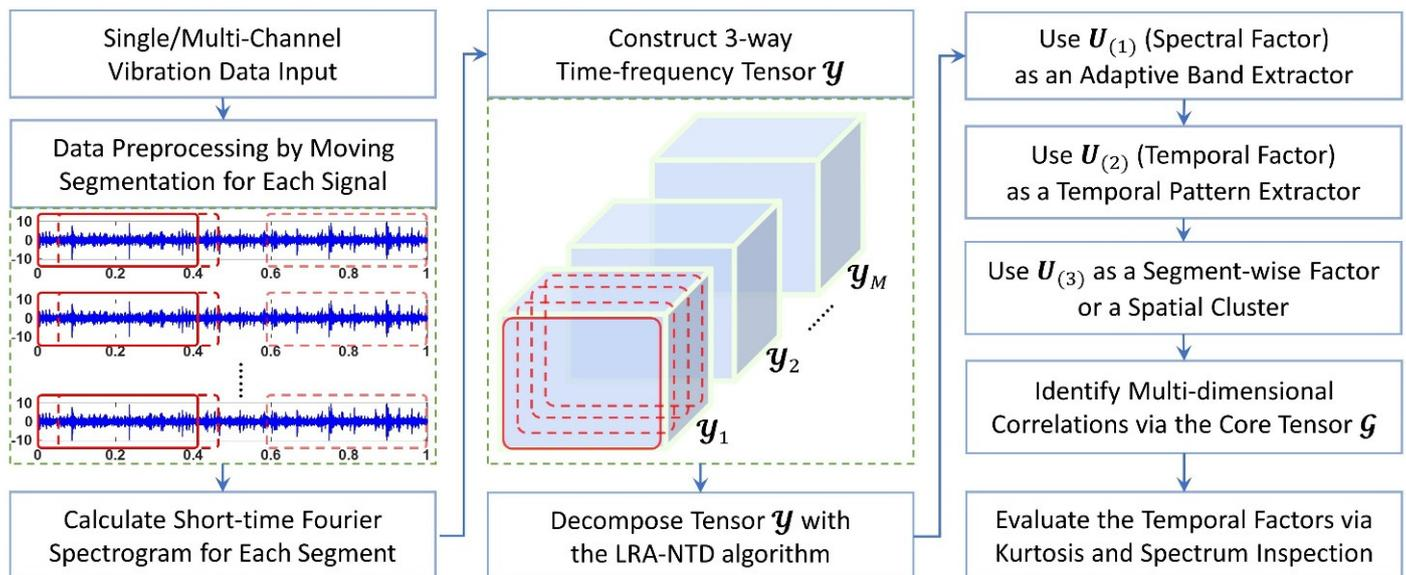
Figure 4. Flowchart of the diagnostic methodology.
