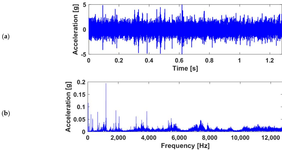
Figure 5. (a) The horizontal acceleration signal and (b) its amplitude spectrum in Case A.
