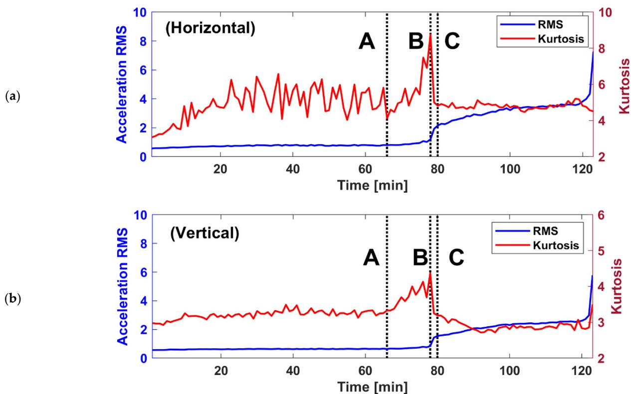
**Figure 2.** Trends of the overall bearing vibration by the acceleration RMS values and Kurtosis: (a) the horizontal-channel vibration and (b) the vertical-channel vibration.
