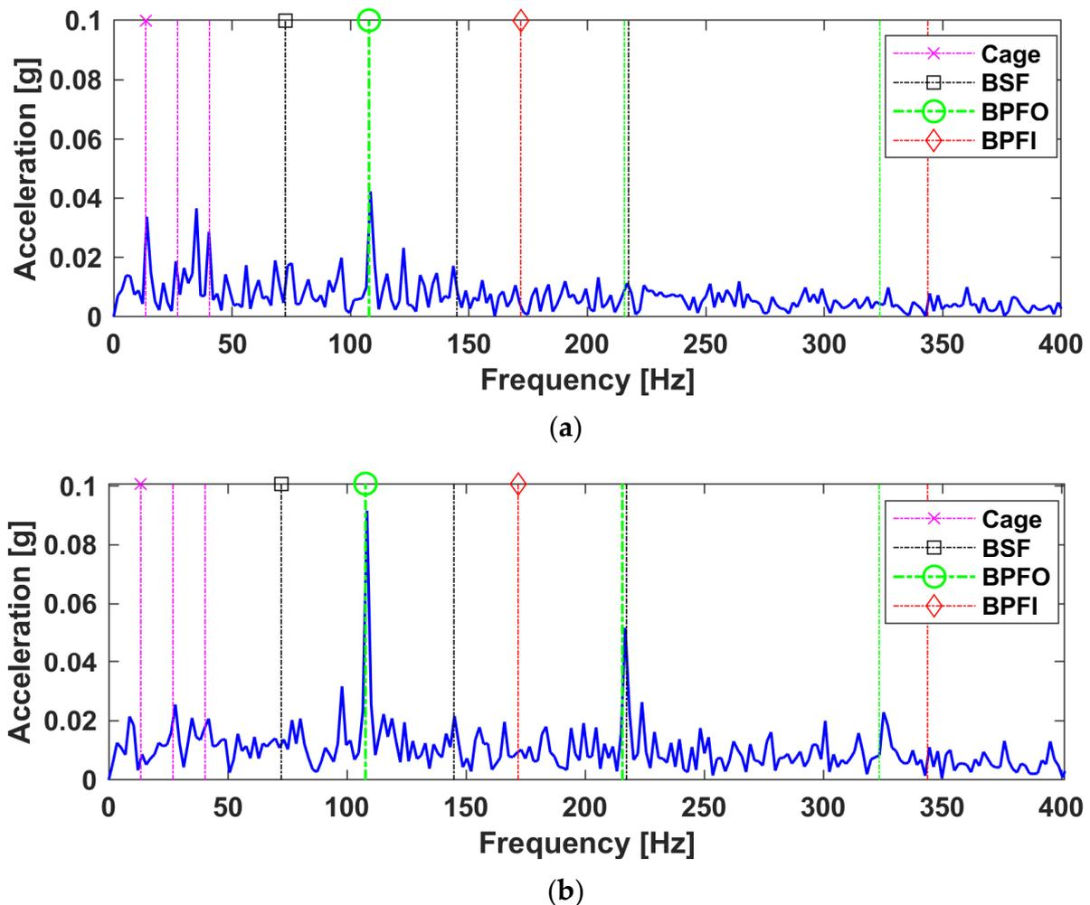
**Figure 11.** Case B results via LRANTD: (a) The amplitude spectrum of TS1 and (b) that of TS2.
