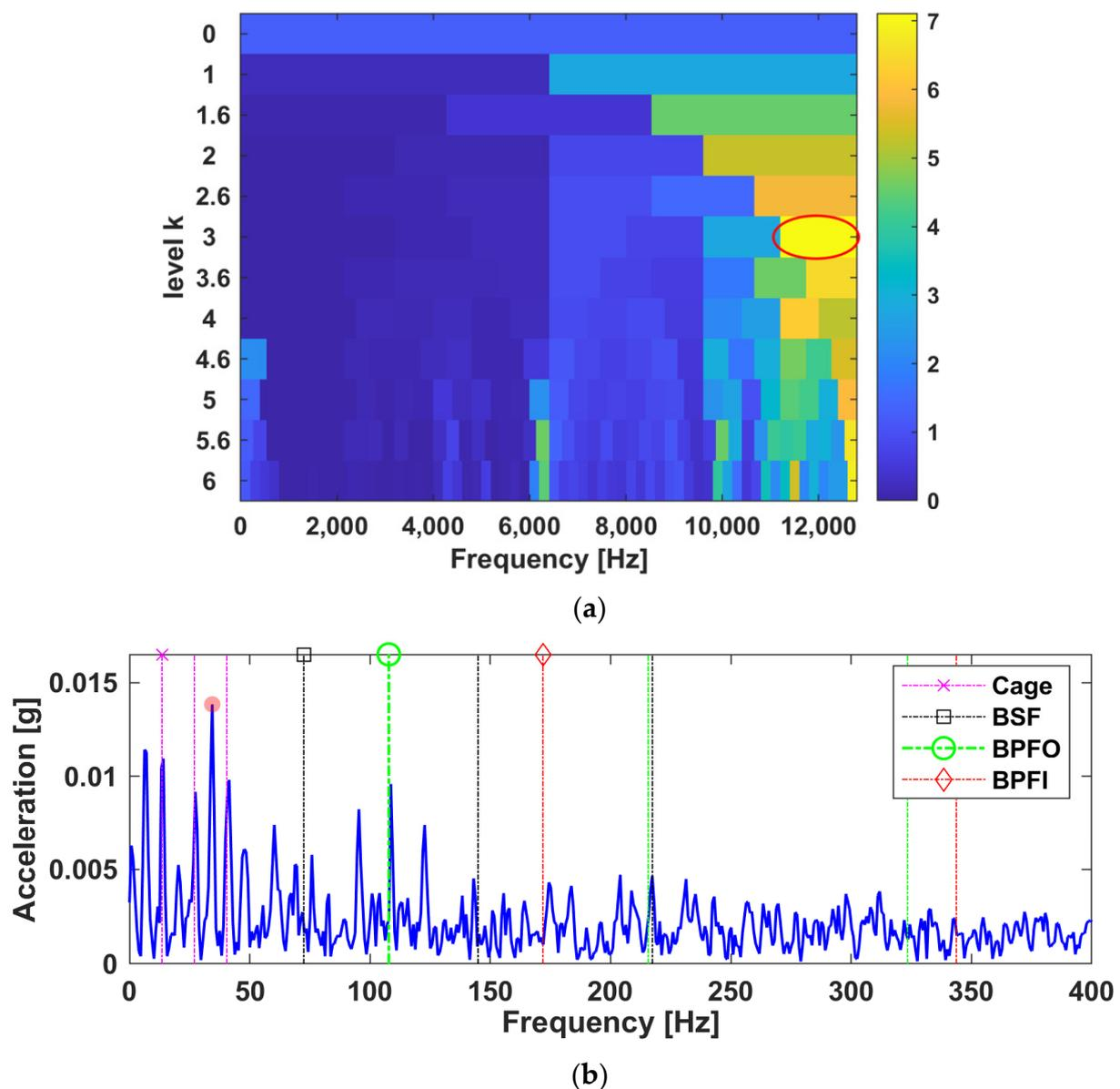
**Figure 17.** Results of Fast Kurtogram: (a) Kurtogram with the maximum kurtosis, 7.1, found at level 3, with band width 1600 Hz, and the central frequency at 12,000 Hz. (b) The envelope spectrum of the filtered signal using the aforementioned optimal filter band.
