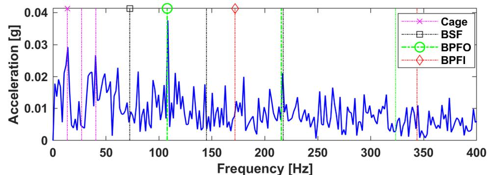
**Figure 8.** Case A result via LRANTD: The amplitude spectrum of TS 4 with clear outer-race fault component.
