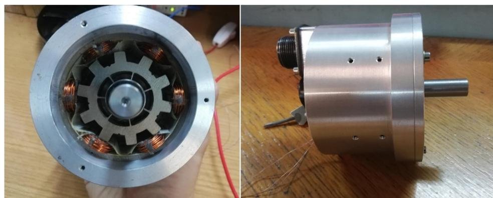
Figure 28. Manufactured prototype. Stator with the windings and rotor are shown on the (left), and complete motor with the housing on the (right) side.
