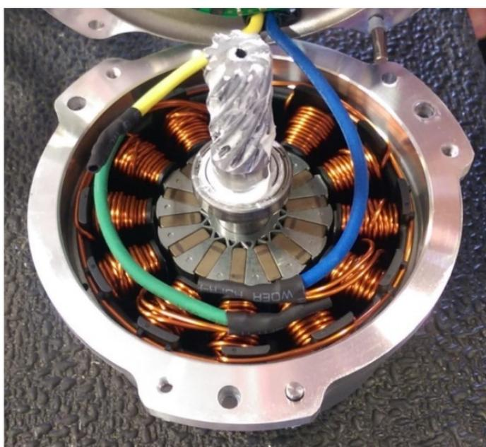
**Figure 1.** IPM from Shimano Steps mid-drive bike system.
