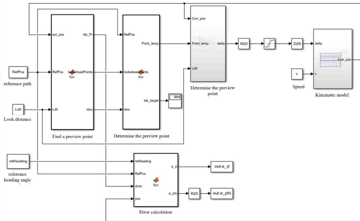
Figure 5. Simulation model of 4WS pure tracking algorithm.
