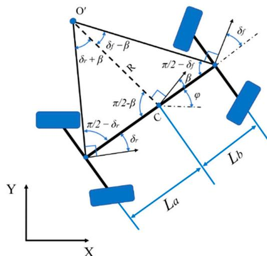
Figure 2. 4WS vehicle kinematics model.
