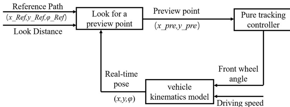
Figure 3. Framework diagram of traditional pure tracking algorithm.
