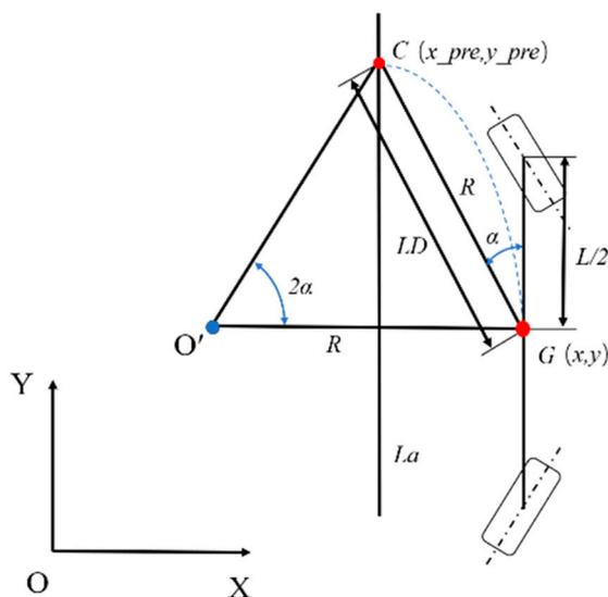
Figure 4. 4WS pure tracking model.
