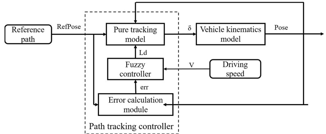
Figure 10. Path tracking simulation flow chart.
